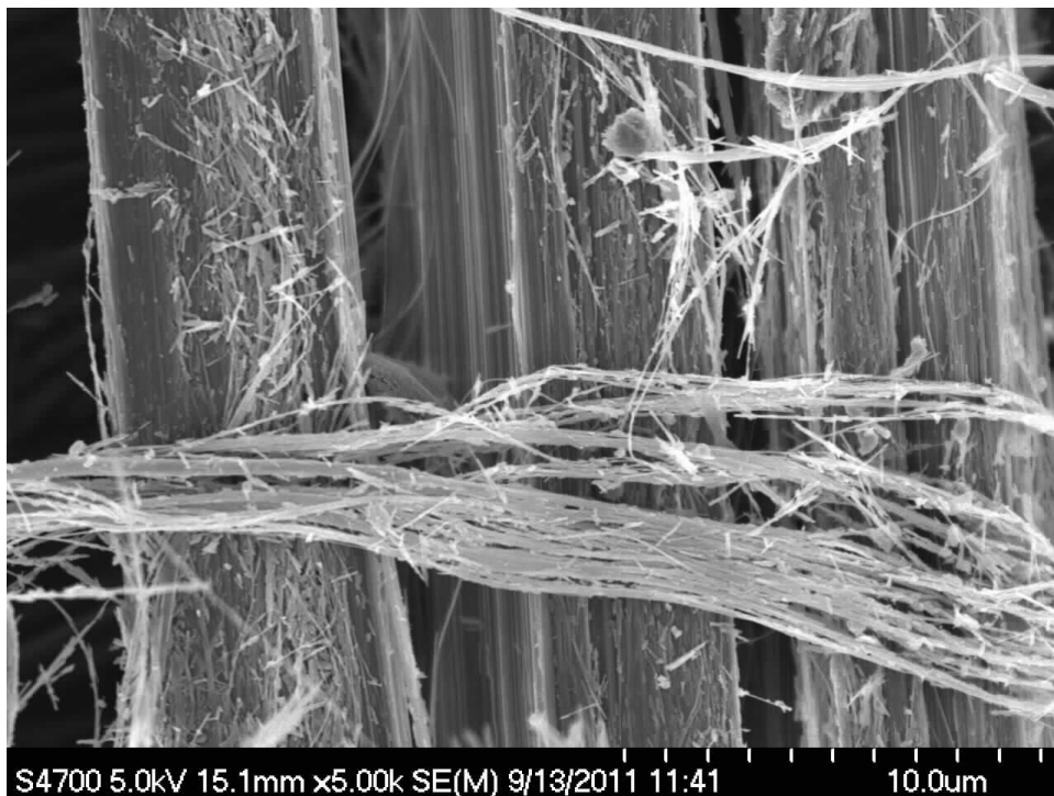
Figure 1.2. FESEM image of chrysotile bundles magnified 3000 times.
