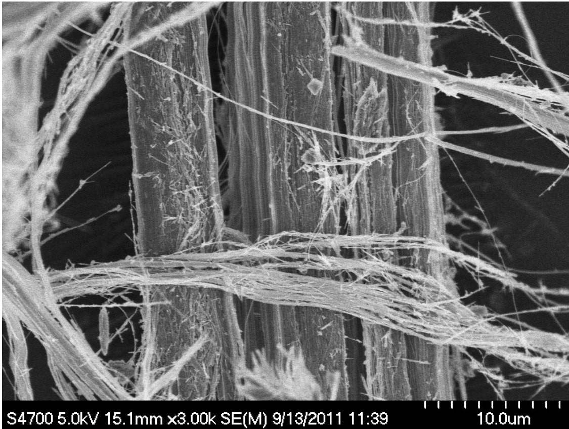
Figure 3.1. FESEM image depicting a bundle of untreated chrysotile fibers magnified 3000X.
