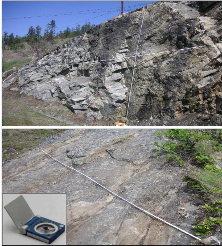
Figure 3.3. Scanlines on a vertical outcrop face (top image) and on the upper orthogonal surface of the outcrop (lower image) at outcrop location 1.
