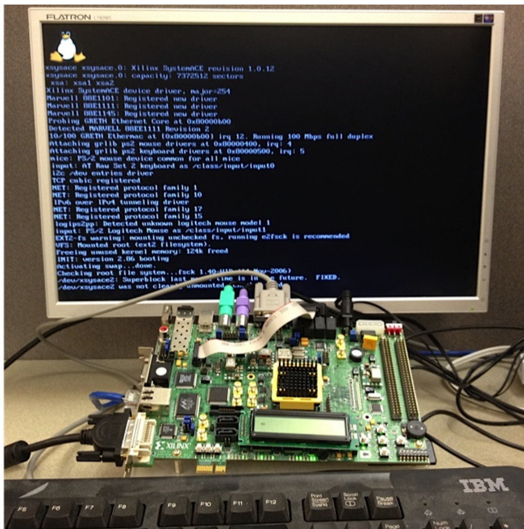
Figure 5.1: LEON3 SoC running on a Virtex-5 FPGA shown booting Linux.
