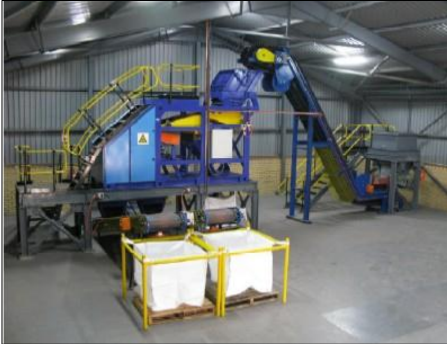
Figure 2-6 The Full-Scale RADOS XRF Ore Sorter Installed at Mintek (Fickling, 2011)
