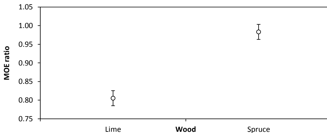
Figure 4.8: Modulus of elasticity (MOE) ratio (MOE bioassayed veneer/MOE sound wood) lime and spruce veneers. Lime veneers incubated with fungi isolated from weathered wood showed a significantly lower MOE ratio than spruce veneers. MOE ratio close to one indicated that MOE was similar to that of sound wood. Error bars correspond to \pm SED
