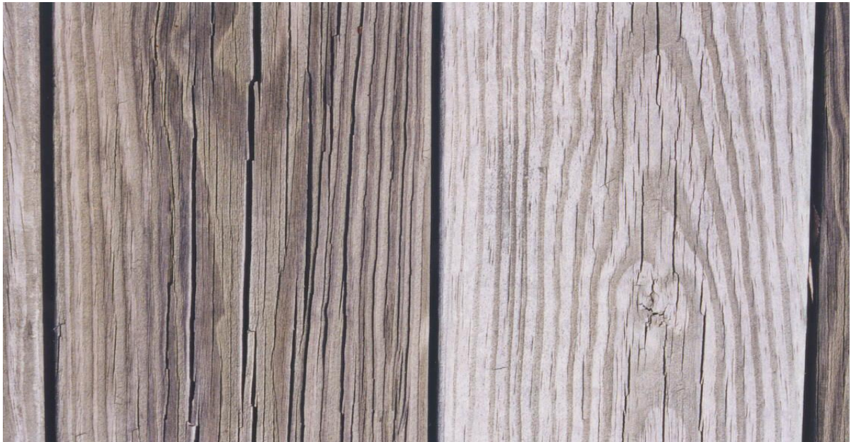
Figure 2.1: Appearance of weathered Southern pine ( Pinus sp.) wood. Note the graying and surface checking of the wood
