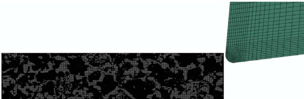
Figure 4.21 FE model of workpiece material with ferrite and pearlite phases.
