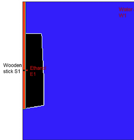
(b) Schematic representation of the thermocouple location (experiment) and monitor points (model) in the cell/domain
