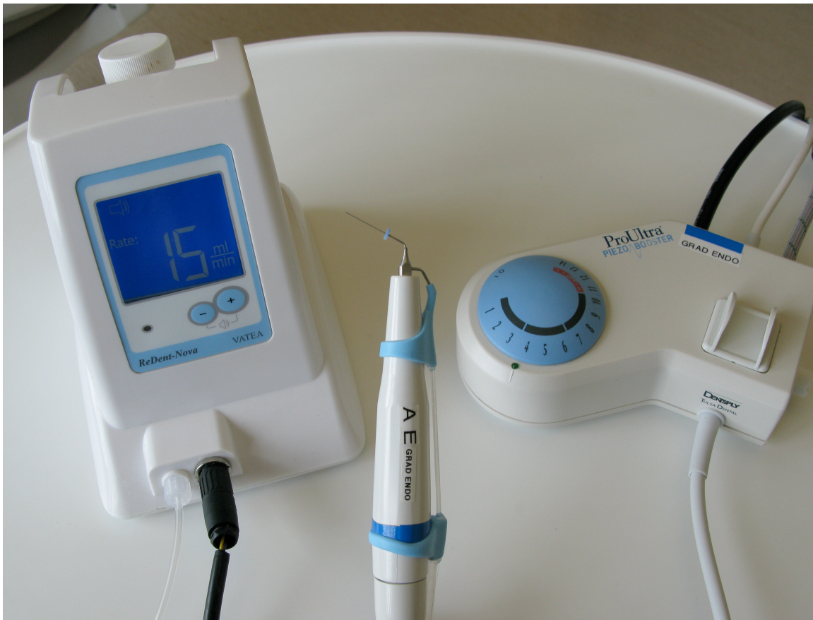
Figure 4. Ultrasonic experimental setup. Ultrasonic unit with handpiece, irrigation delivery unit, and VPro StreamClean Ultrasonic Needle.
