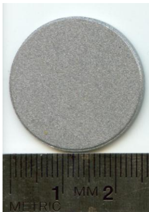
Figure 3.2: Porous SS430 metal substrate
