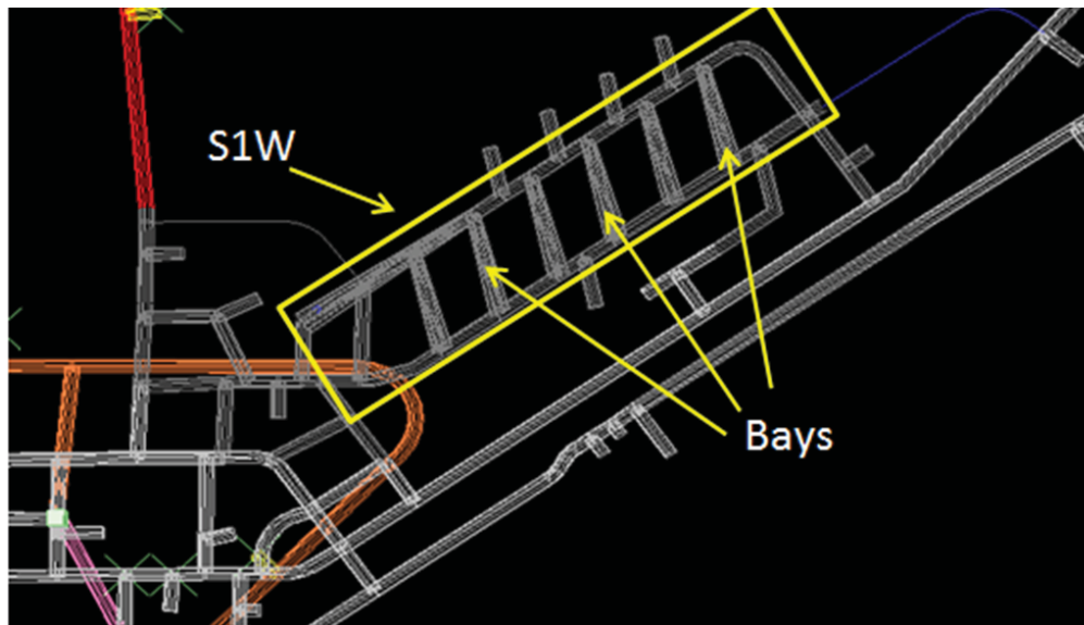
Figure A.4.18. Tested Shaft 1 Workshop Bays Massive Excavation
