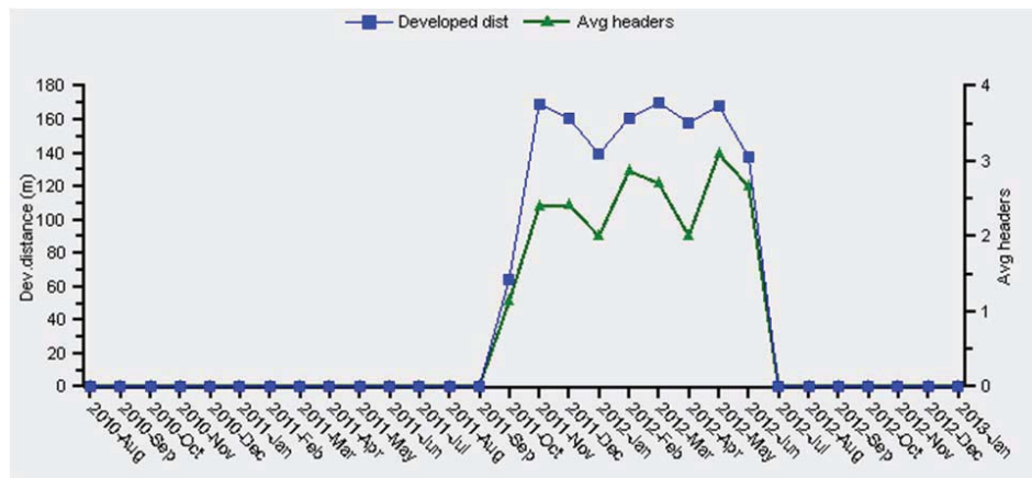
Figure A.4.19. Monthly Development Meters and Available Headings of Mine Area 31
