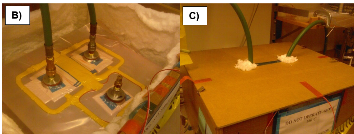
Figure 3.3. Heated in-plane permeability setup. A) Lay-up order of consumables, and direction of in-plane gas flow; B) Setup within heating enclosure; C) Setup during heated permeability testing.
