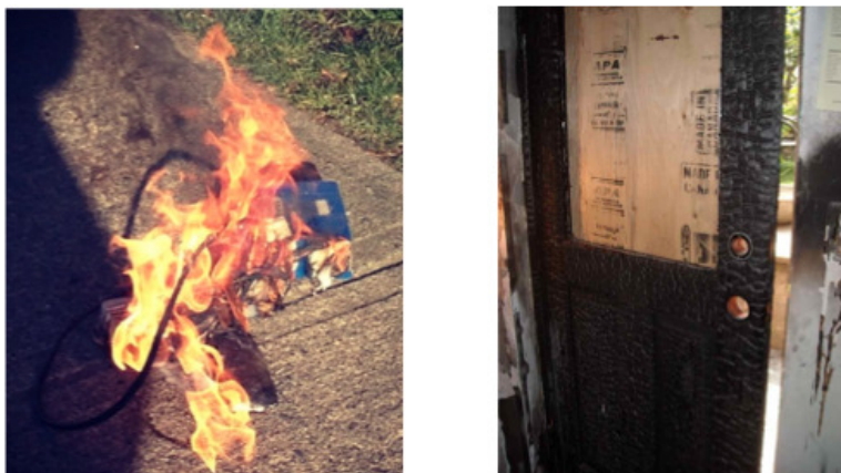
Figure 1.2: Batteries with flammable electrolyte can cause serious fire and damage and are a key motivator in the development of solid polymer electrolytes as an alternative to conventional liquid and gel electrolytes. (left) Three flaming 24 V flaming polymer gel battery packs that began combusting during use on an electric bicycle. (right) The remains of the author’s door after a house fire caused by a 36 V lithium manganese battery and charger.
