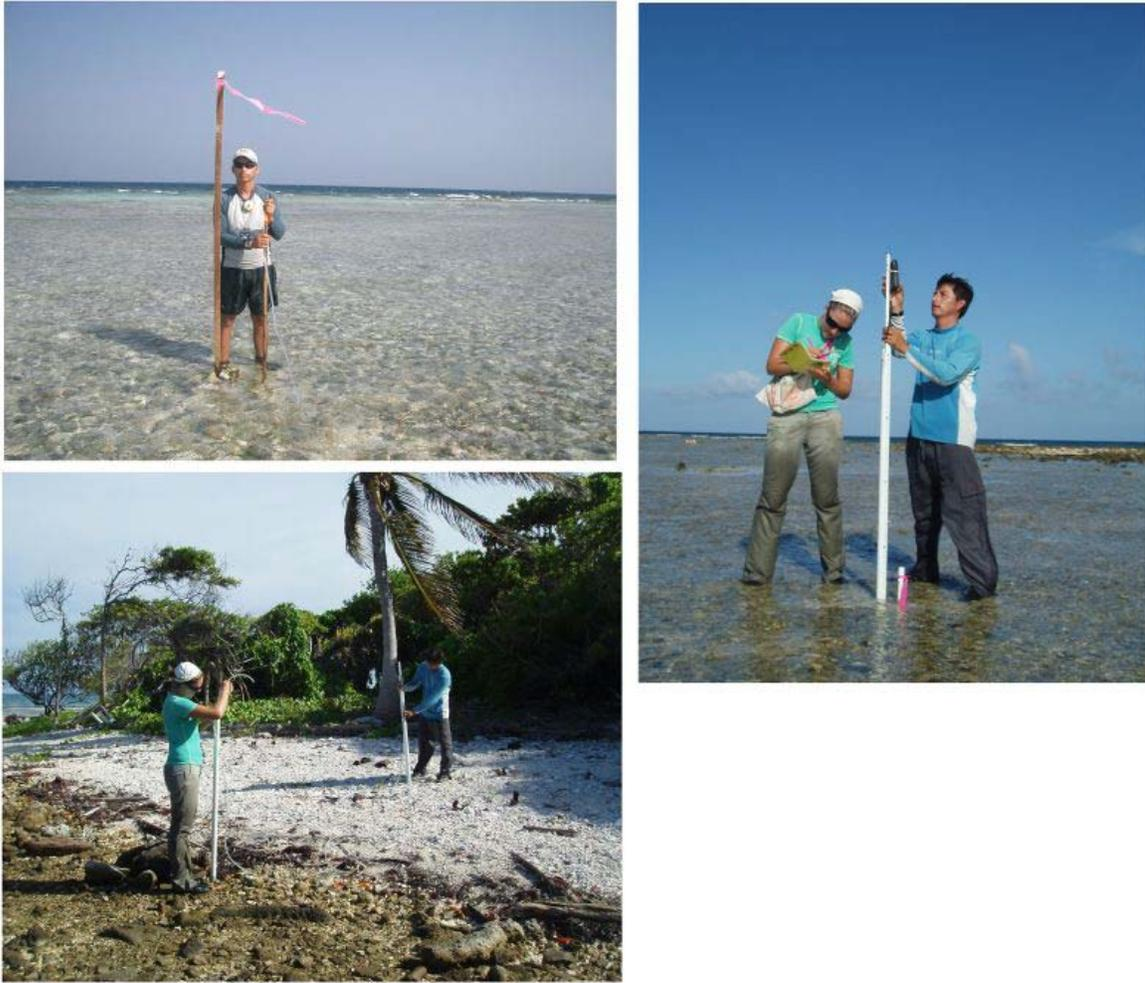
**Figure N.1.** A 15 m length clear tube with a 1 cm inside diameter was used along with two graduated telescoping poles, and GPS, to measure substrate elevation.
