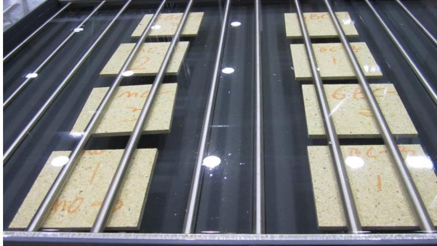
Figure 3.8: Thickness swell samples in the tank.
