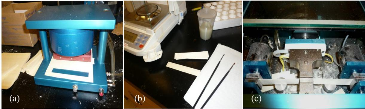
Figure 3.2: (a) air-operated clipper, (b) applying resin, (c) automatic bond evaluation system.
