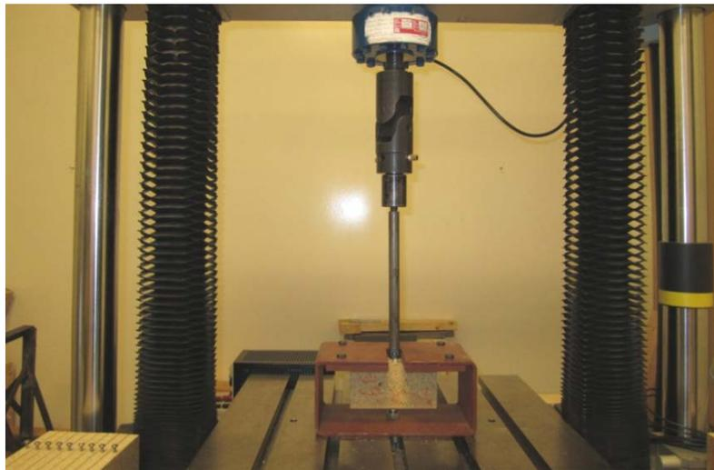
Figure 3.6: The assembly for edge screw withdrawal test
