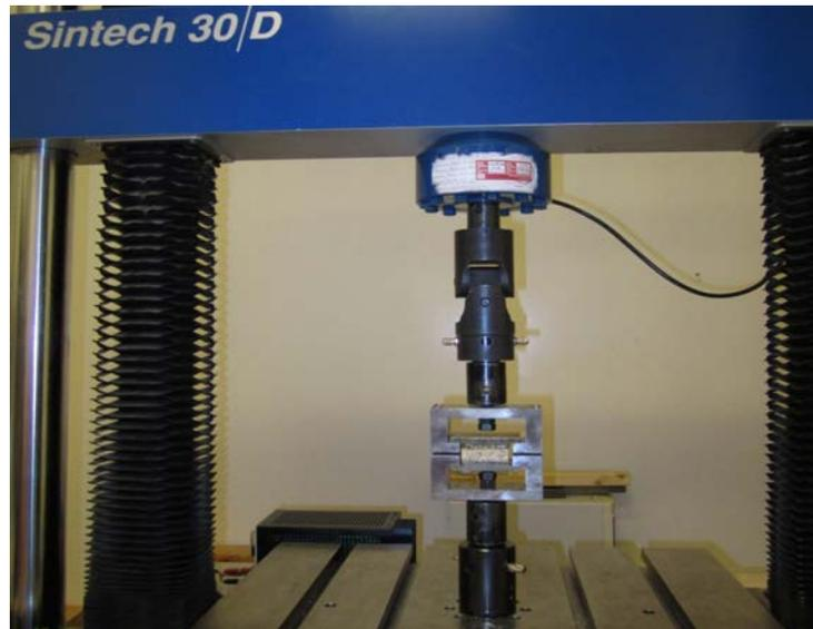
Figure 3.7: The assembly of internal bonding (IB) test
