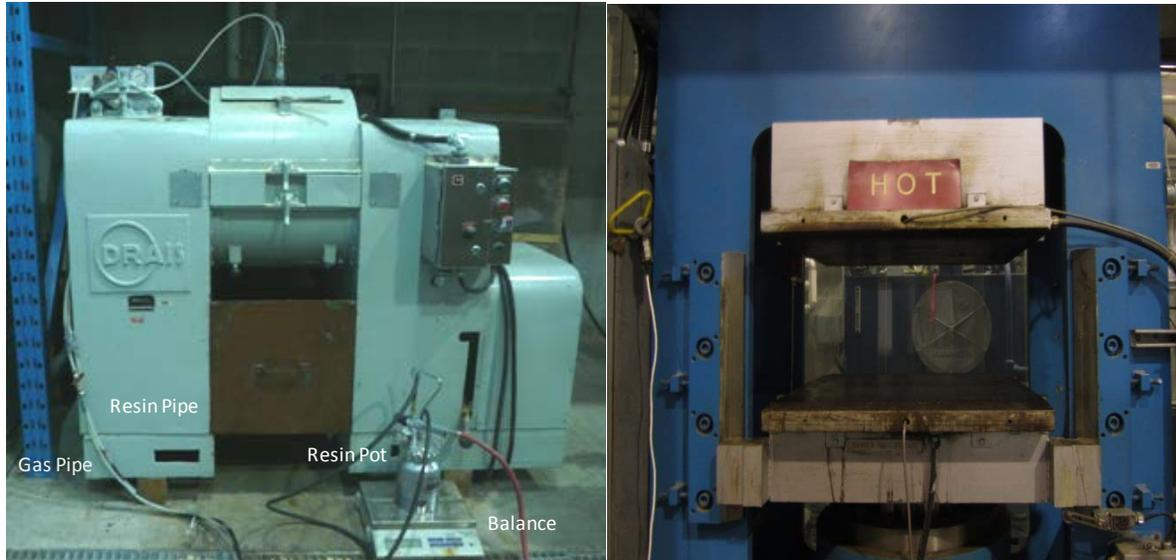
Figure 3.3: (left) Drais particleboard batch-blender and (right) Pathex press.
