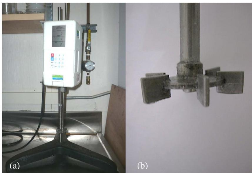
Figure 3.1: The Labmaster TS-2010 mechanical mixer: (a) the mixing head and (b) the impellor agitator.
