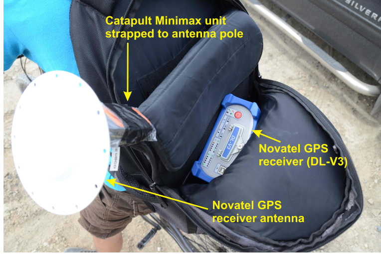
Figure 4.11: Catapult Minimax unit strapped to the Novatel GPS receiver antenna pole. [Photograph by Darren Handschuh]
