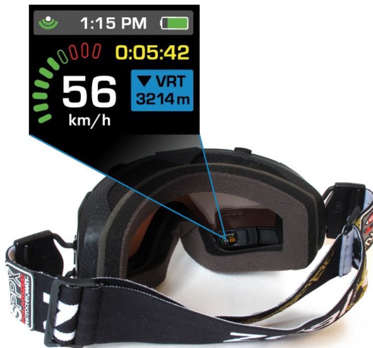
Figure 1.3: Micro-LCD display in Recon Action Sports Goggles [1].
