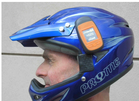
Figure 4.10: Catapult Minimax unit affixed to the biker’s helmet.
