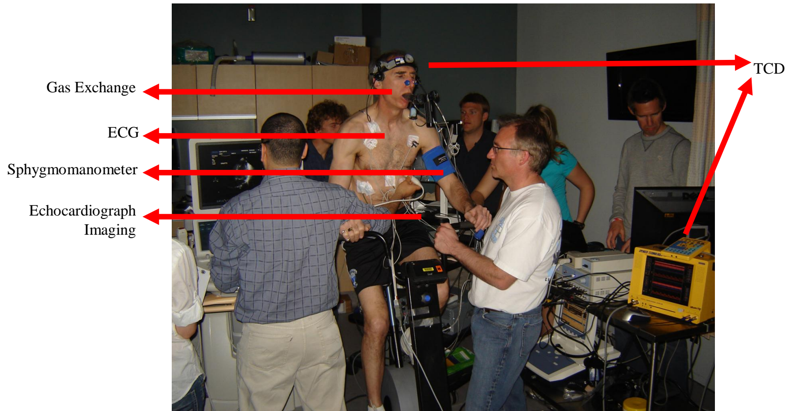
Figure 3.1. Instrumentation setup on subject during the incremental cycling exercise protocol. Transcranial Doppler ultrasound (TCD), Electrocardiograph (ECG).
