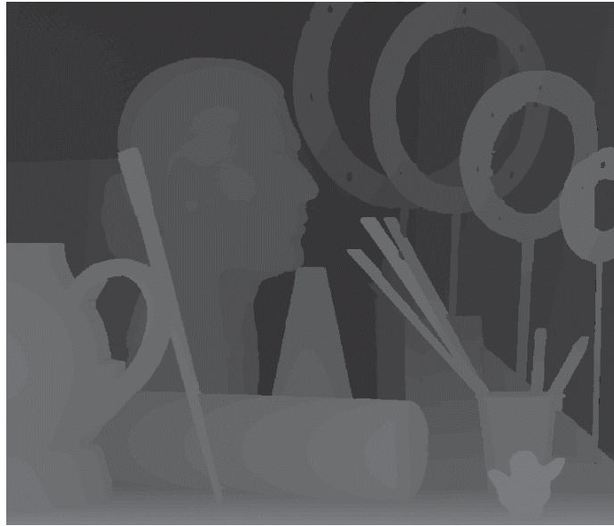
Figure 4.5 Reference disparity map obtained using input images of the same exposure: Arts
