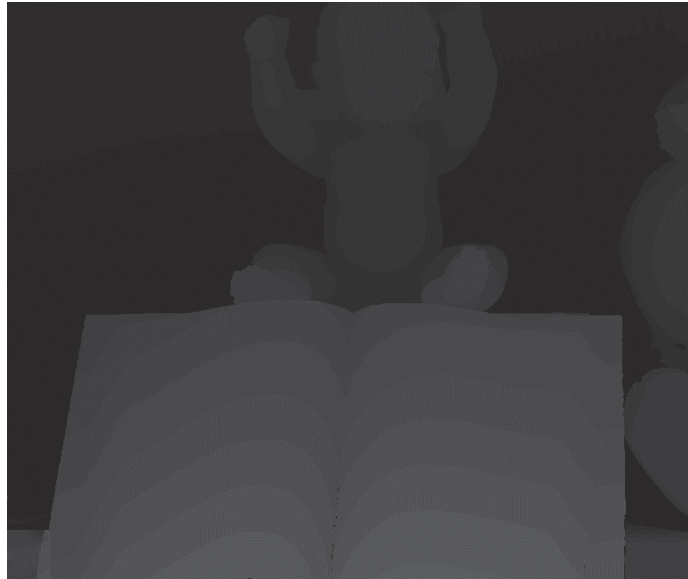
Figure 4.7 Reference disparity map obtained using input images of the same exposure: Baby
