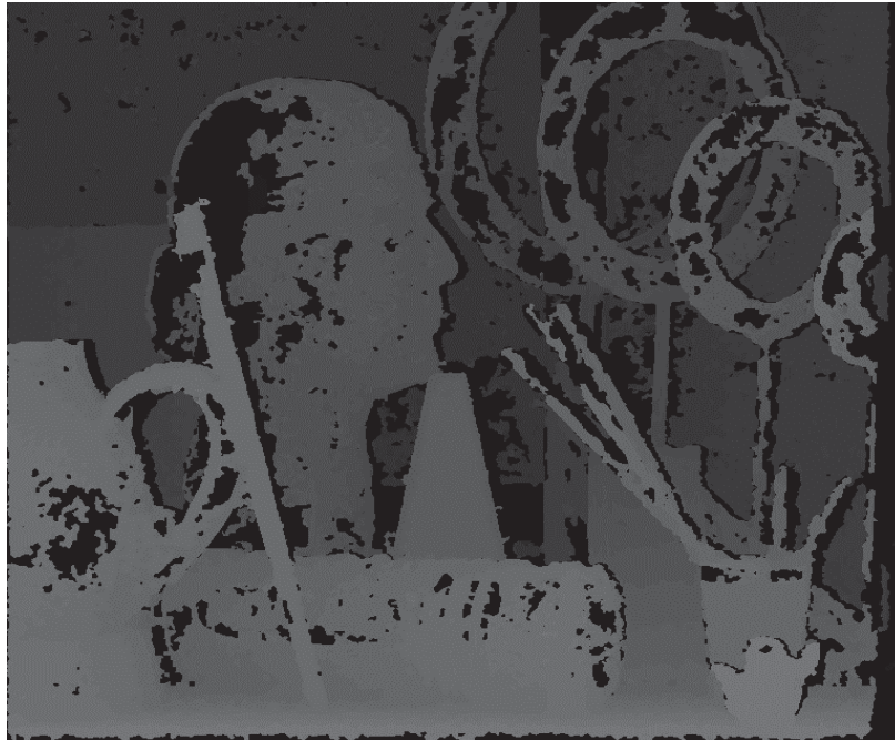
Figure 3.8 Initial disparity map obtained by our algorithm after running step 1: Arts
