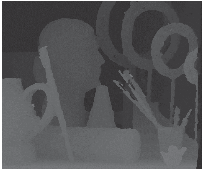
Figure 4.6 The final disparity map obtained using our algorithm: Arts. The disparity map is generally accurate and smooth except at the edges of different objects and the pencils. This is because it is very difficult to completely remove the fattening effect caused by using a window based cost function in stereo matching.
