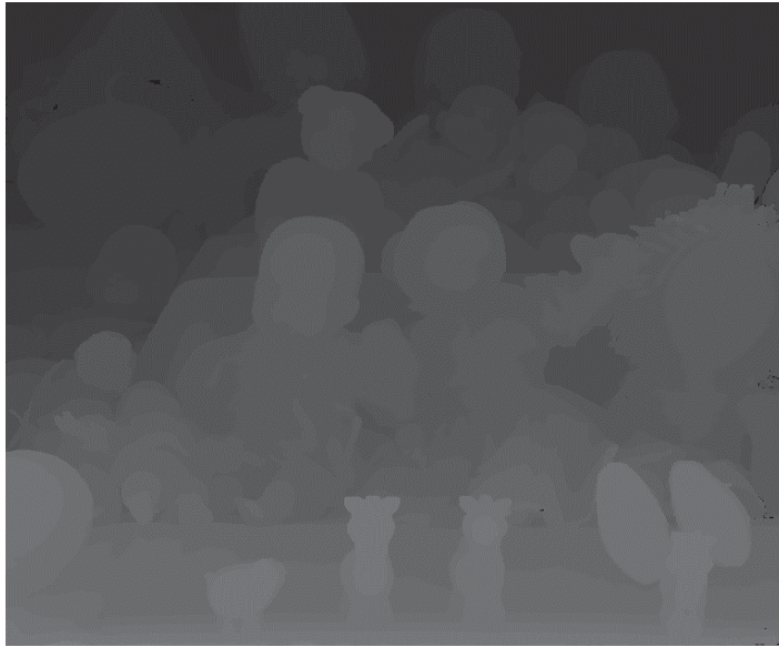
Figure 4.3 Reference disparity map obtained using input images of the same exposure: Dolls
