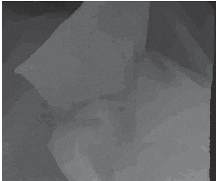
Figure 4.2 The final disparity map obtained using our algorithm: Clothes. The values at the erroneous pixels in the initial disparity map are successfully obtained by the refinement step. This is because the saturated regions in the input images are small and scattered.
