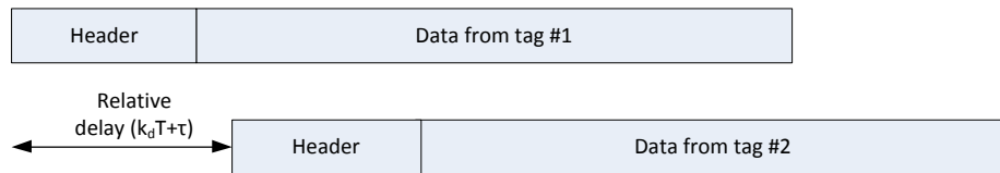
Figure 7.1: The known header is used to detect the beginning of a new packet and estimate the relative delay k_d
