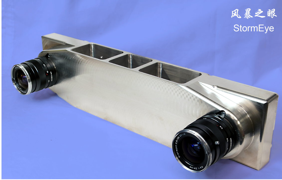
Figure 1.4: Prototype of the real-time position sensing system based on stereo-vision
