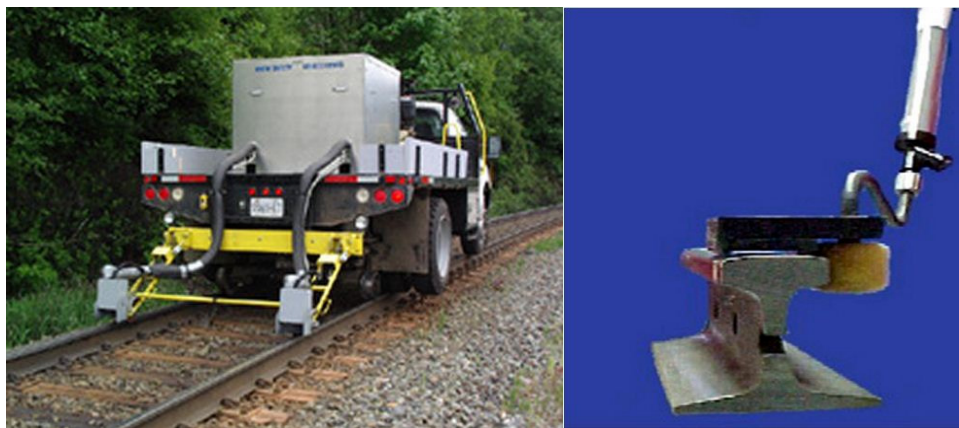
(a) HiRail Vehicle mounted TOR Friction Control System (b) Liquid LCF Gauge Face Lubricant
