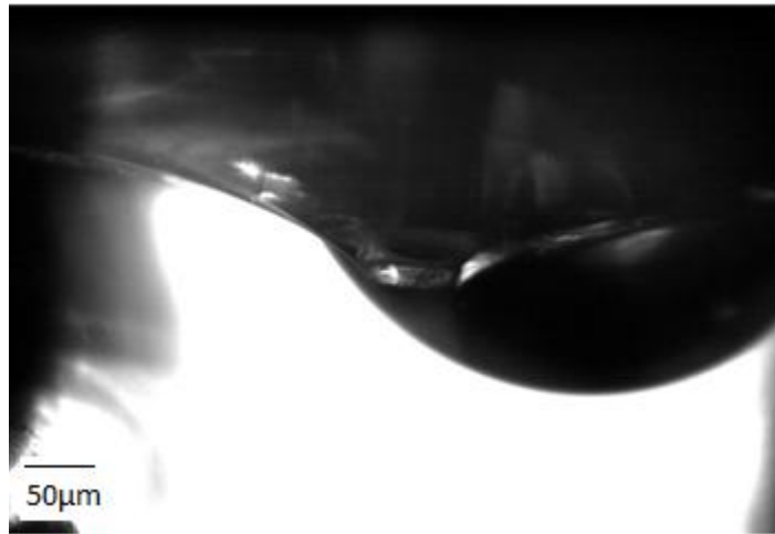
Figure 5.17 Total wetting of the surface resulted from low kinetic energy and high internal pressure
