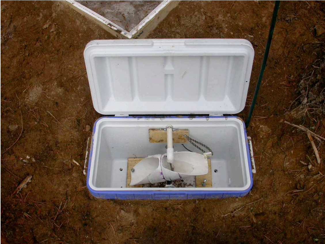
Figure 2.10. Tipping bucket mechanism for the snowmelt lysimeter shown in Figure 2.9.
