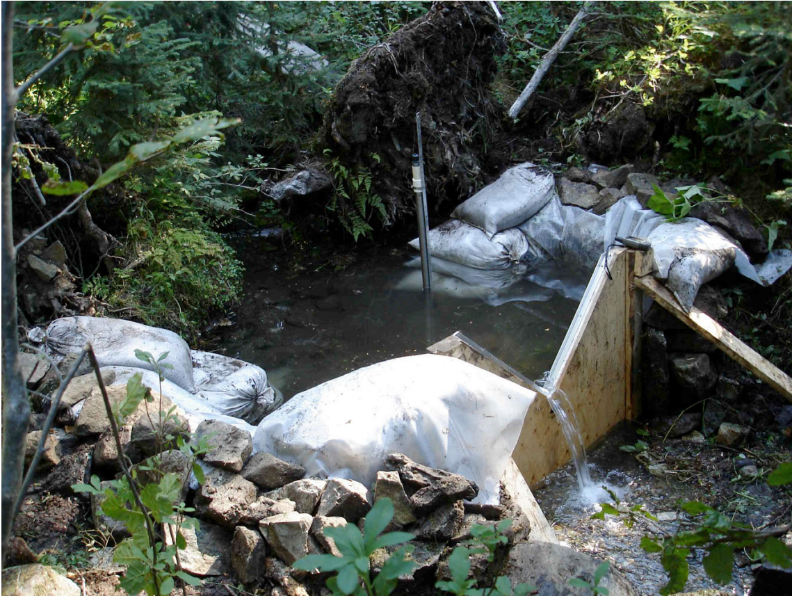
Figure 2.11. Streamflow site with a 90° v-notch wier and a stilling well.
