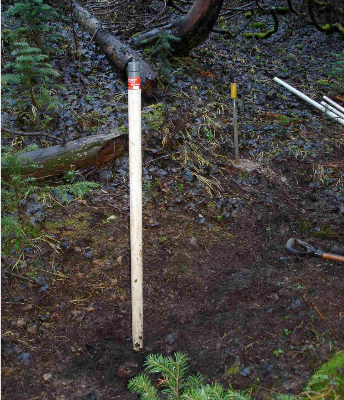
Figure 2.7. Hillslope site showing a PVC groundwater well (lower) and an epoxy access tube for manually measuring soil saturation using an AquaPro capacitance soil moisture sensor (upper).
