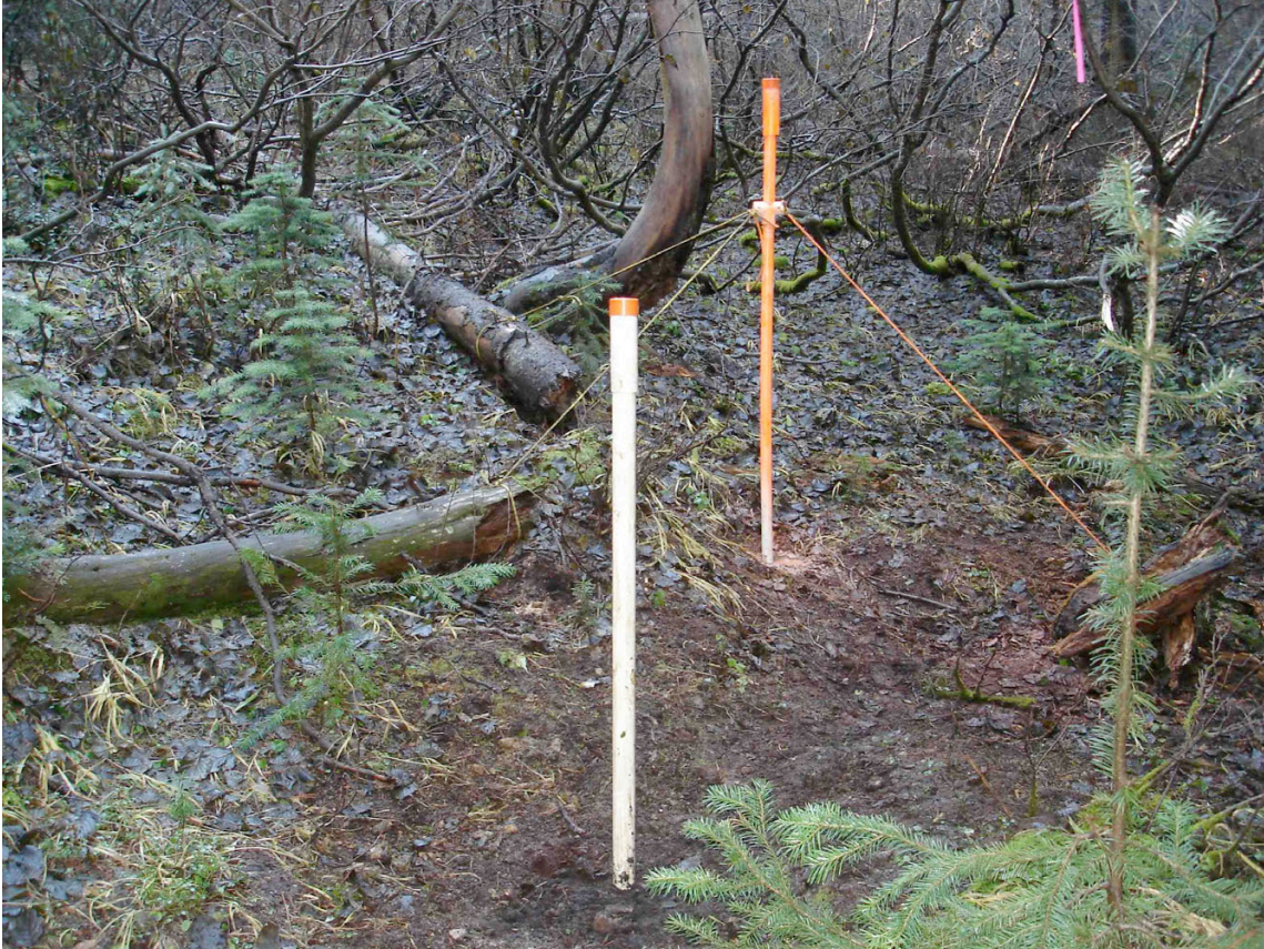
Figure 2.8. Groundwater well and epoxy access tube from Figure 2.7 with a PVC extension added to the access tube to allow measurement of soil saturation while snow-covered.
