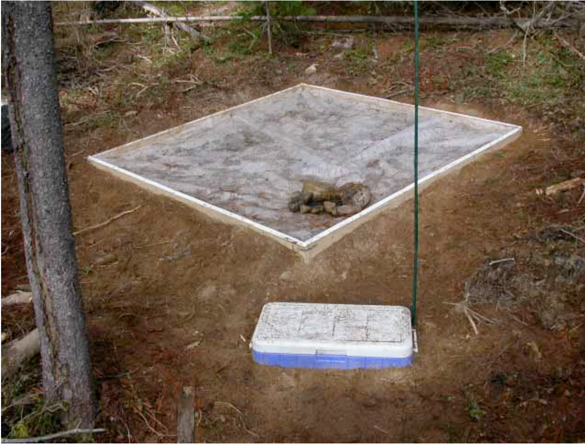
Figure 2.9. Snowmelt lysimeter lined with 10 mil polyethylene, an outlet drain (surrounded by rocks to help keep a mesh debris filter in place), and a cooler box containing a tipping bucket mechanism for measuring lysimeter outflow.
