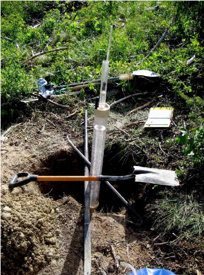
Figure 2.12. Hydraulic conductivity test in operation using a Guelph Permeameter.
