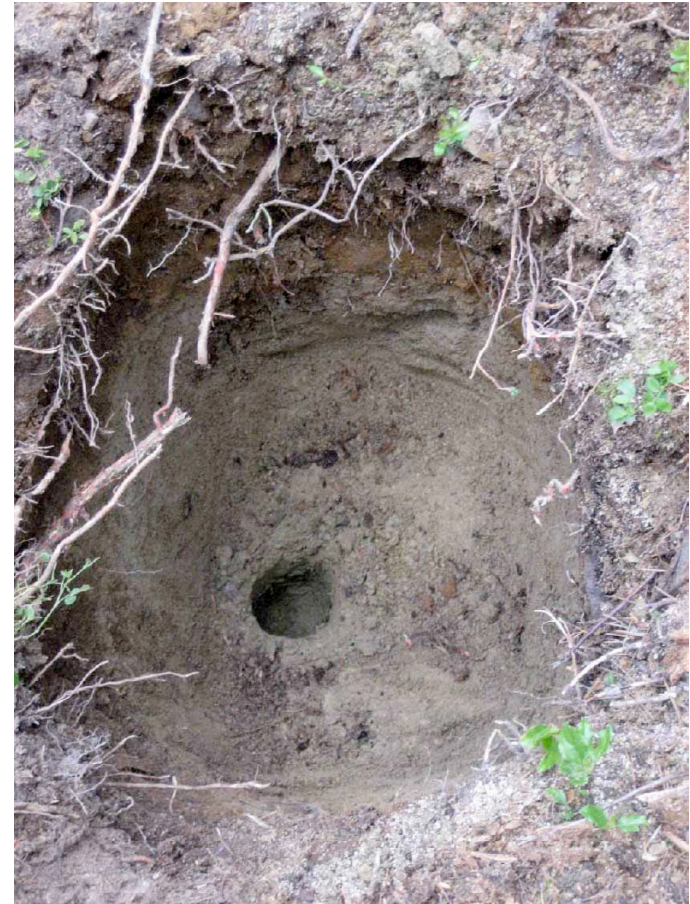
Figure 2.13. Bore-hole prepared for a hydraulic conductivity test using a Guelph Permeameter.
