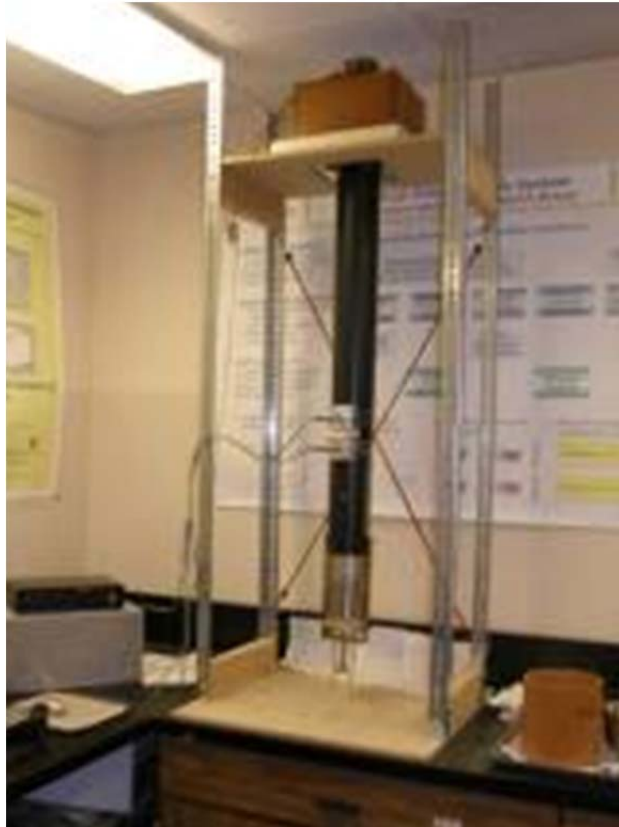
Figure 2 Impedance tube experimental set-up
