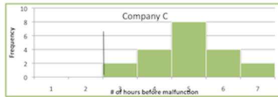
(c) Data from Company C \bar{x}_C = \bar{x}_B , \sigma_C = \sigma_B , and N_C = 2N_B
