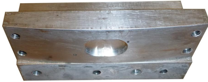
Figure 24: Specimen holder. Note the curvature on the front where the specimen mount and the slot machined out to allow for the thin case assumption.
