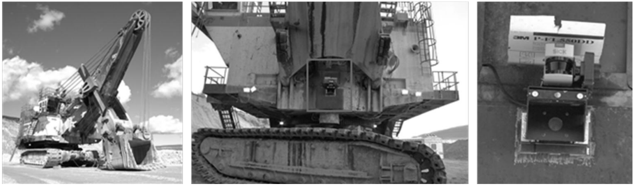
Figure 4-21: Laser Scanner and Camera Setup on a Mining Rope Shovel
