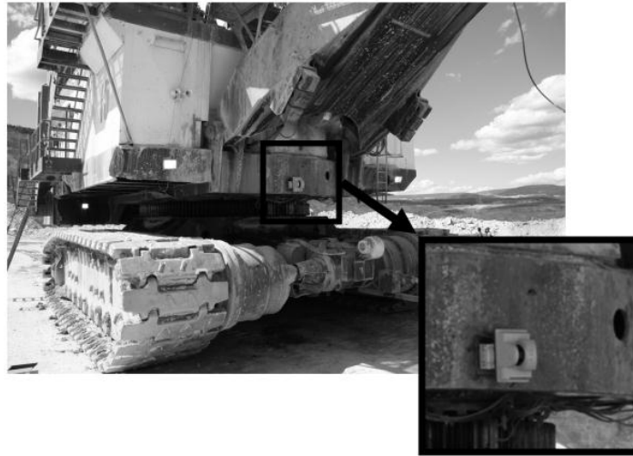
Figure 3-12: Vertical Installation of a Laser Scanner Underneath the Shovel Boom
