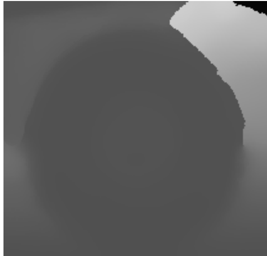
Figure 4-26: An Example of the Edge-Blur in a Depth Image Obtained by the Yang Method
