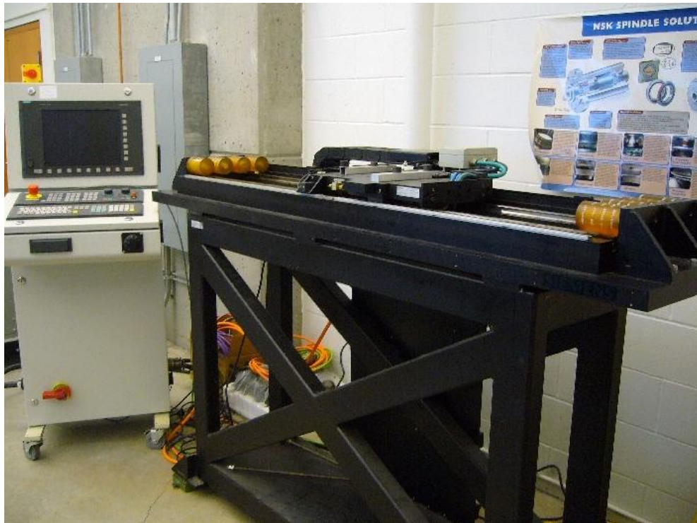
Figure 3.3: Siemens Linear Motor and the SIMODRIVE 611U
