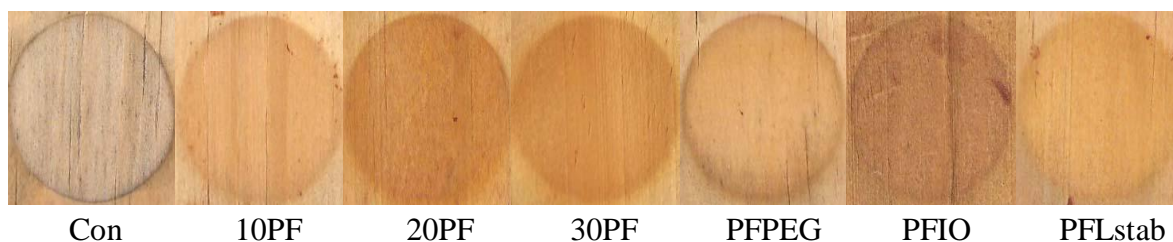
Figure 4.19 Appearance of treated radiata pine specimens after 2000 hours of natural weathering (The circular areas inside the specimens were exposed to natural weathering, whereas the areas outside the circles were covered by metal masks. Con = Control; 10PF = 10% PF resin; 20PF = 20% PF resin; 30PF = 30% PF resin; PFPEG = 10% PF resin + 10% Polyethylene glycol; PFIO = 10% PF resin + 1% Iron oxide; PFLstab = 10% PF resin + 2% Lignostab)
