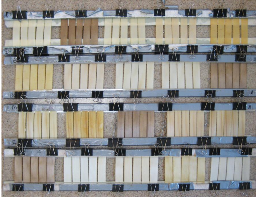
Figure II.3 Veneers treated with different additives (10% Lignosulphonate, 10% PEG, 1% iron oxide, 2% lignostab 1198)
