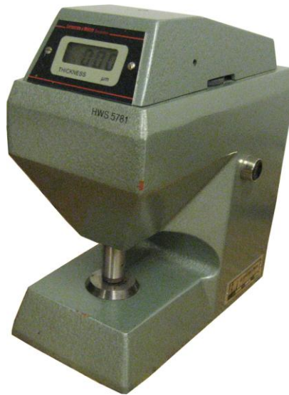
Figure 4.3 Digital micrometer used to measure the thickness of individual wood veneers
