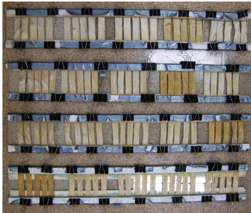
Figure II.3 Veneers treated with different additives (10% Lignosulphonate, 10% PEG, 1% iron oxide, 2% lignostab 1198)
