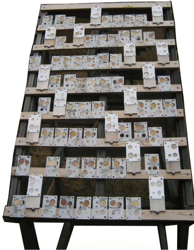
Figure 4.8 Weathering rack containing treated wood composite specimens
