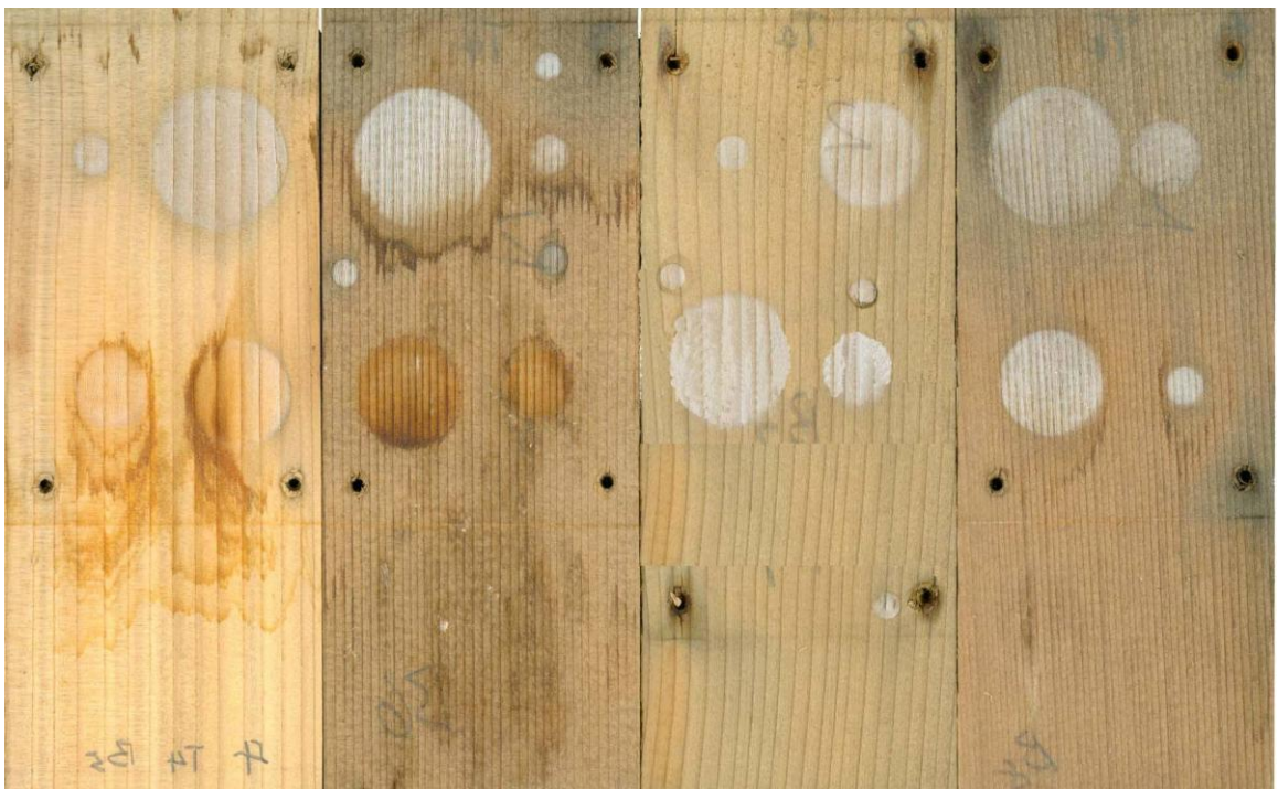
Figure I.8 Western red cedar specimens exposed in QUV weatherometer for 1000 hours
