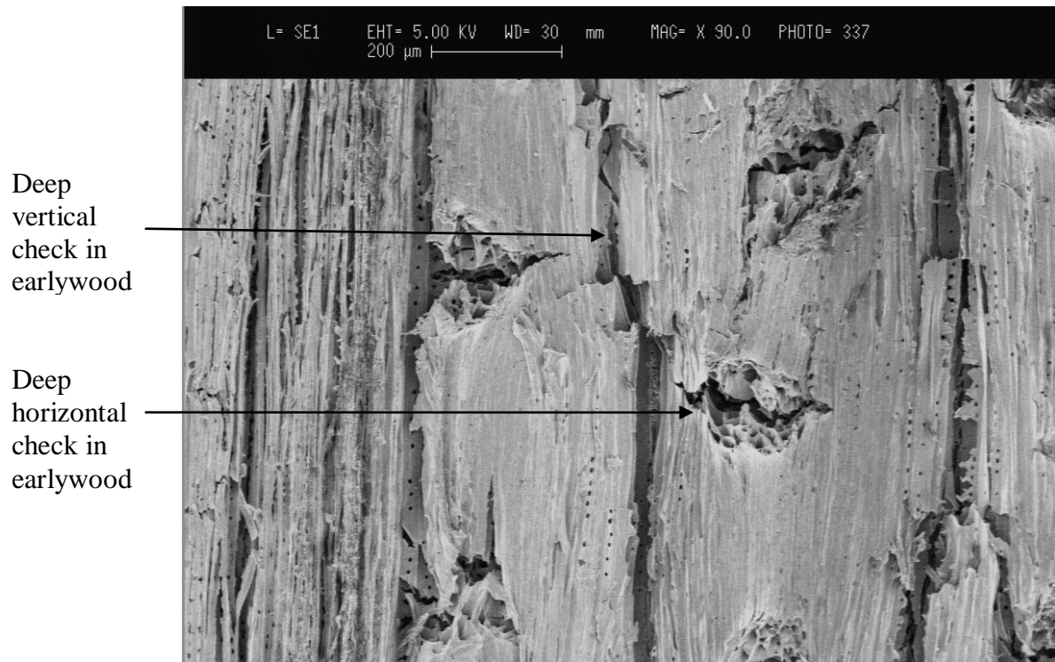
Figure 3.22 Micro-structural changes at the surface of a western red cedar specimen exposed in a xenon-arc weatherometer for 500 hours
