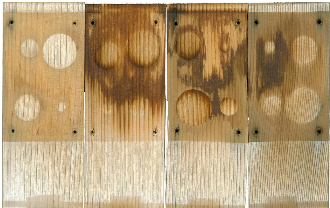
Figure 1.12 Western red cedar specimens exposed in xenon arc weatherometer for 1000 hours
