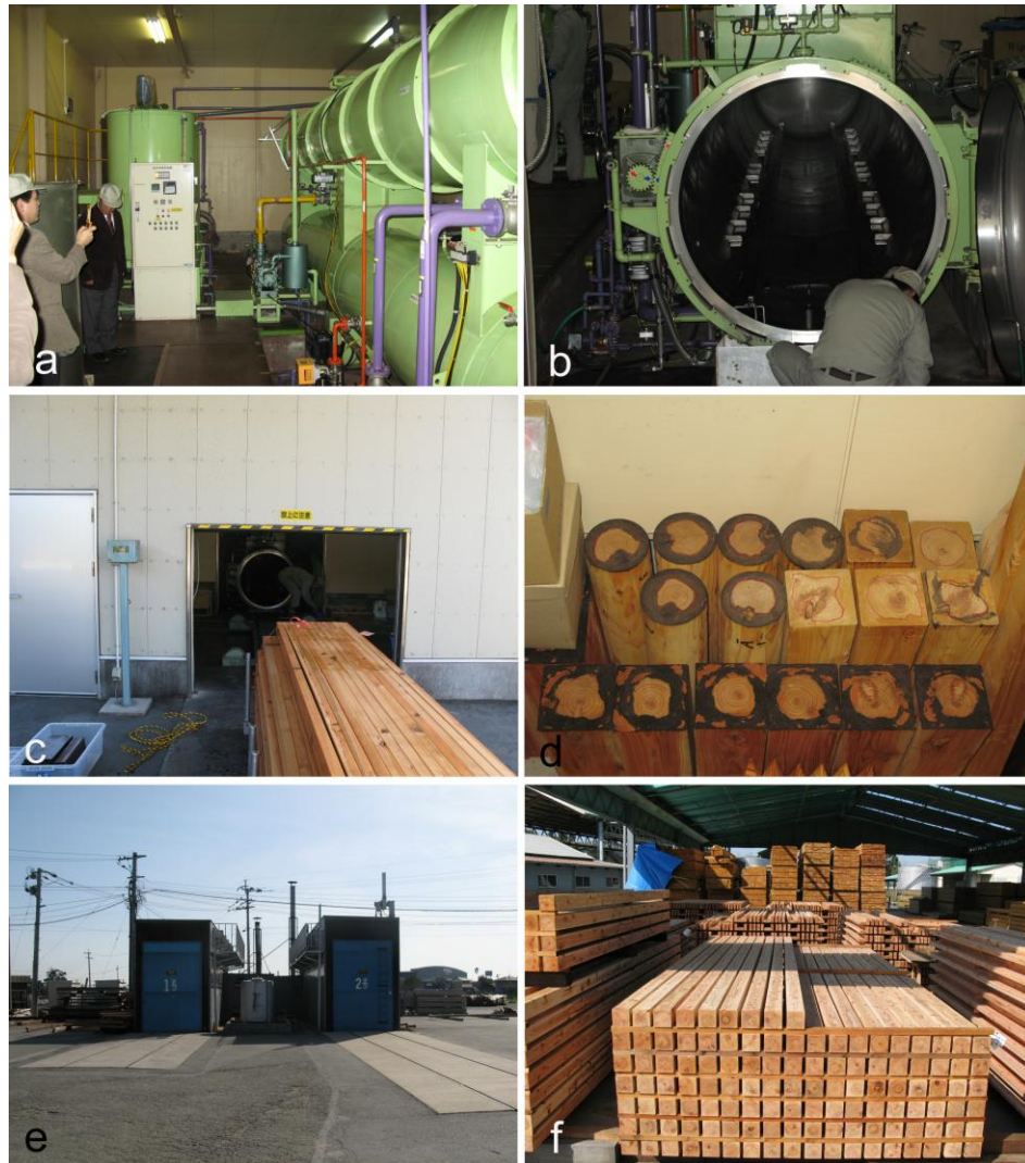
Figure 2.17 Process used to manufacture phenol formaldehyde impregnated wood at Kyushu Mokuzai a, Pressure treatment cylinder and tank in back-ground (left) used to store chilled PF resin; b, Inside of pressure treatment cylinder; c, Charge of timber after treatment with PF resin. Note the excess PF resin solution on treated Japanese cedar; d, Penetration of PF resin into Japanese cedar timber; e, Kilns used to cure the timber treated with PF resin; f, PF-treated timber air drying after treatment (Mokuzai Gakkaishi. http:// www.kyumoku.co.jp )
