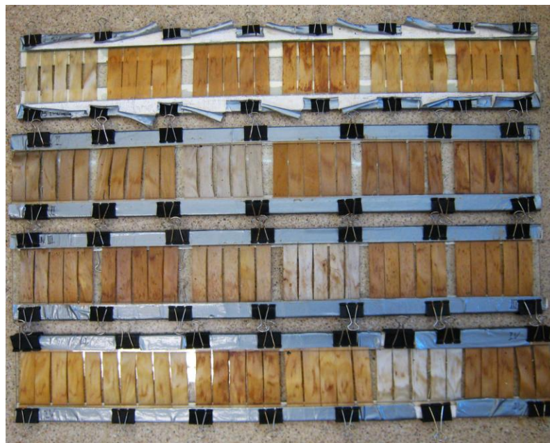
Figure II.6 Veneers treated with 12% PF rein, 12% PF resin containing different additives (10% Lignosulphonate, 10% PEG, 1% iron oxide, 2% lignostab 1198) after 50 days natural weathering
