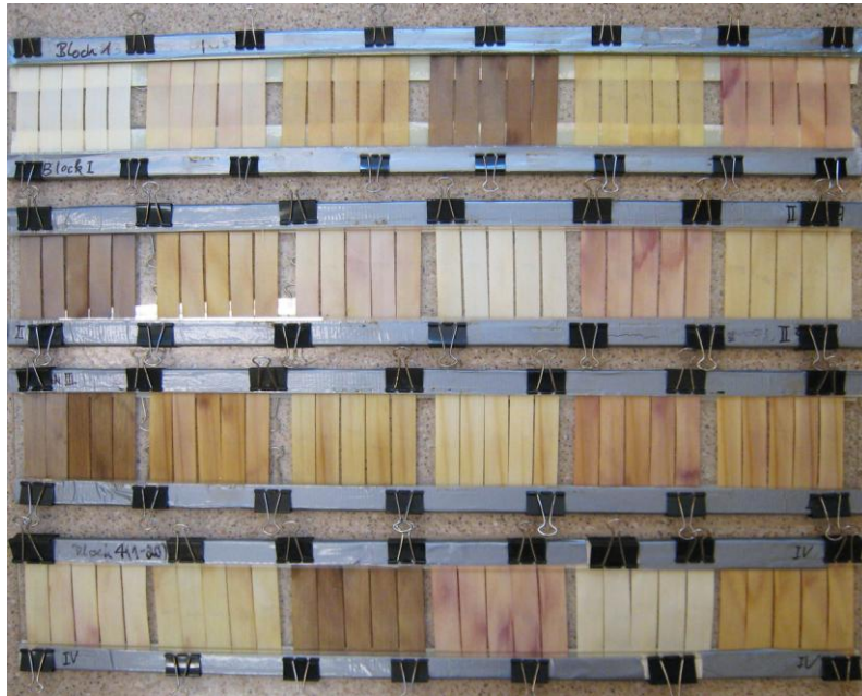
Figure II.5 Veneers treated with 12% PF rein, 12% PF resin containing different additives (10% Lignosulphonate, 10% PEG, 1% iron oxide, 2% lignostab 1198)
