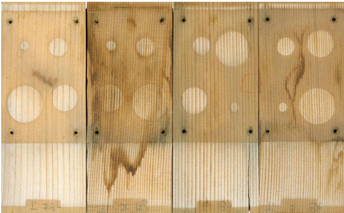
Figure I.10 Western red cedar specimens exposed in xenon arc weatherometer for 250 hours
