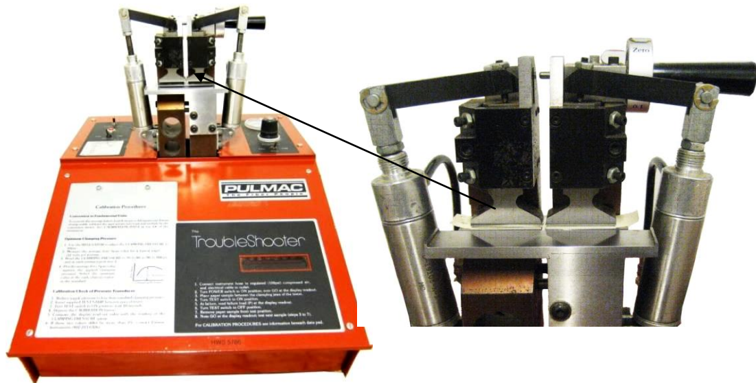
Figure 4.9 Pulmac TS 100 paper testing machine used to measure the zero-span tensile strength of thin wood veneers (left) and a close-up of the jaws of the testing device (right)
