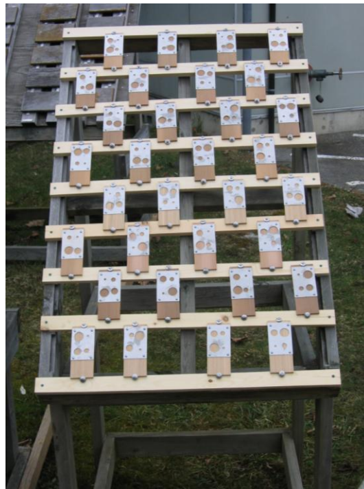
Figure 3.4 Rack containing the masked western red cedar specimens that were exposed to natural weathering
