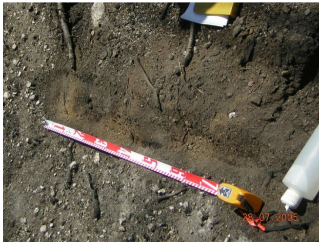
Figure 3-6: Water being dribbled from a squeeze bottle along a shallow ‘trench’ across the slope to determine the Spatial Repellency Index
