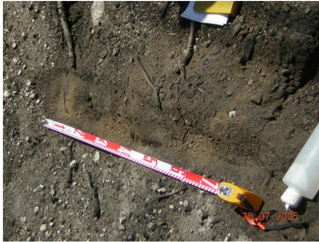
Figure 2-6: Water being dribbled from a squeeze bottle along a shallow ‘trench’ across the slope to determine the Spatial Repellency Index
