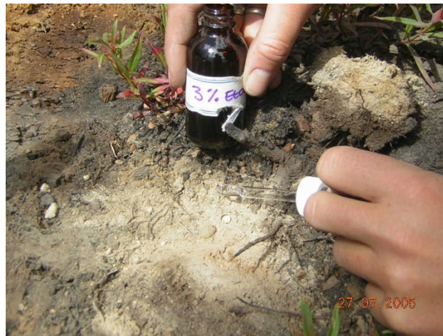
Figure 2-4: The Concentration of Ethanol Drop test showing a drop of ethanol solution beading on the soil surface
