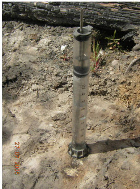
Figure 3-5: A Mini-Disk Infiltrator in the field. The top chamber is adjustable for different tensions
