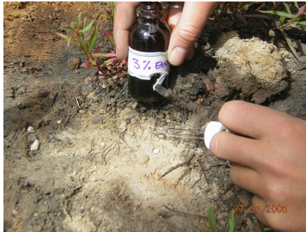
Figure 3-4: The Concentration of Ethanol Drop Test showing a drop of ethanol solution beading on the soil surface
