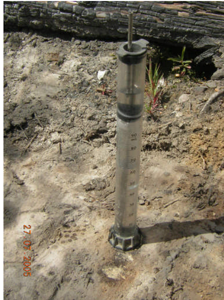
Figure 2-5: A Mini-Disk Infiltrator in the field. The top chamber is adjustable for different tensions
