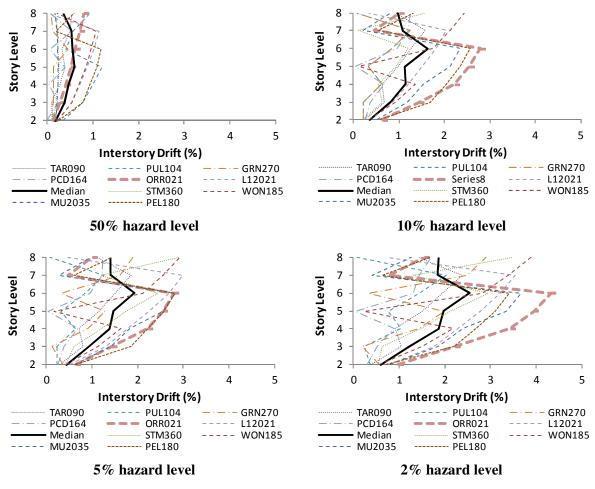
Figure 3.9. Inter-storey drift for retrofitted case with steel bracing
