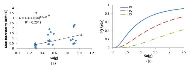
Figure 3.16. Base isolation retrofitting, a) probabilistic seismic demand model, and b) seismic fragility curve
