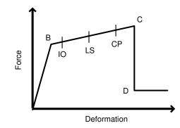
Figure 3.6. Force-deformation response of non-degrading plastic hinge properties (reproduced from FEMA 356 (2000))
