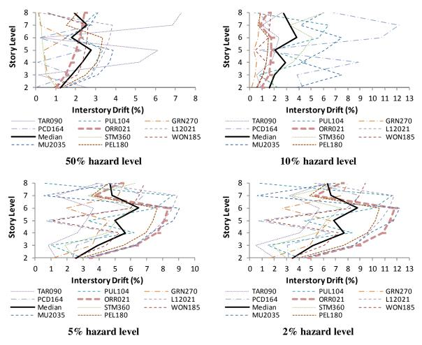
Figure 3.8. Inter-storey drift for unretrofitted case
