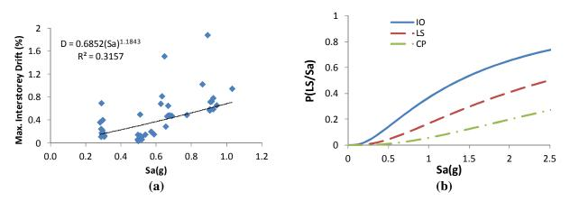
Figure 3.15. Shear wall retrofitting, a) probabilistic seismic demand model, and b) seismic fragility curve
