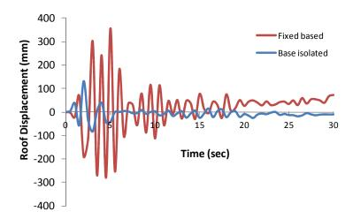
Figure 3.11. Comparison of roof displacement for base-isolated and fixed base model
