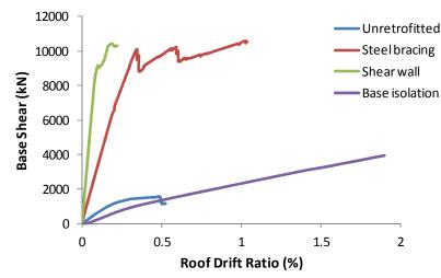
Figure 3.7. Comparison of pushover analysis for unretrofitted and retrofitted cases
