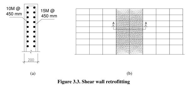
(a) reinforcement detailing of shear wall section, (b) shear wall added to middle bays
