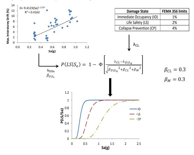
Figure 3.13. Development of fragility model for unretrofitted structure
