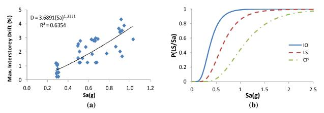
Figure 3.14. Steel bracing retrofitting a) probabilistic seismic demand model, and b) seismic fragility curve
