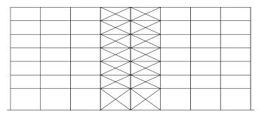
Figure 3.2. Steel bracing retrofitting at the middle bays
