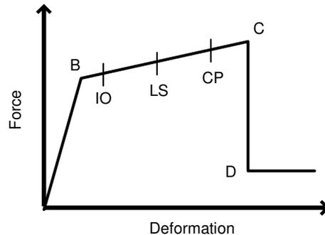
**Figure 3.6. Force-deformation response of non-degrading plastic hinge properties (reproduced from FEMA 356 (2000))**
