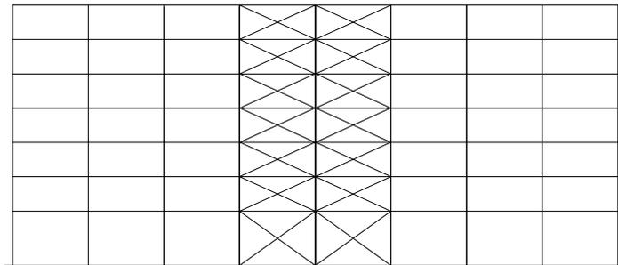
**Figure 3.2. Steel bracing retrofitting at the middle bays**
