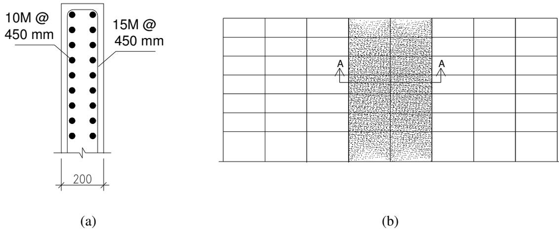
**Figure 3.3. Shear wall retrofitting**
