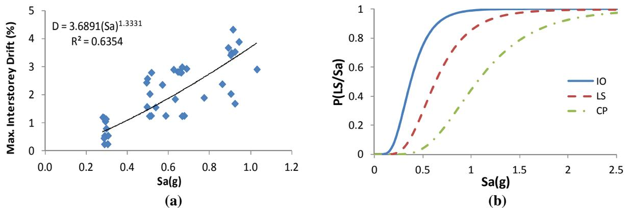
**Figure 3.14. Steel bracing retrofitting a) probabilistic seismic demand model, and b) seismic fragility curve**
