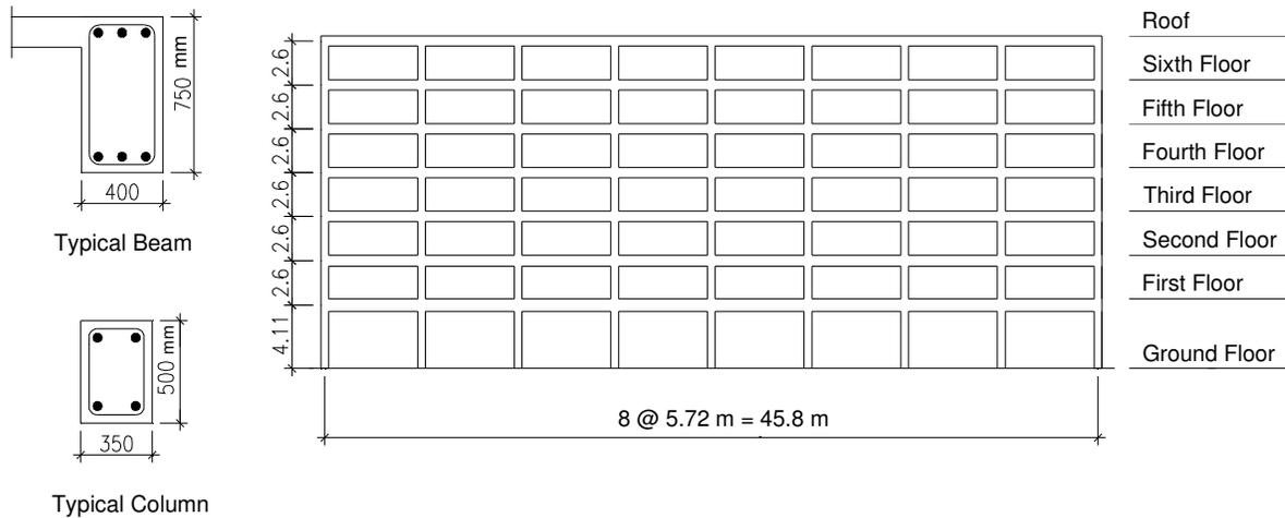
**Figure 3.1. Elevation view and typical section detailing of the case study frame**
