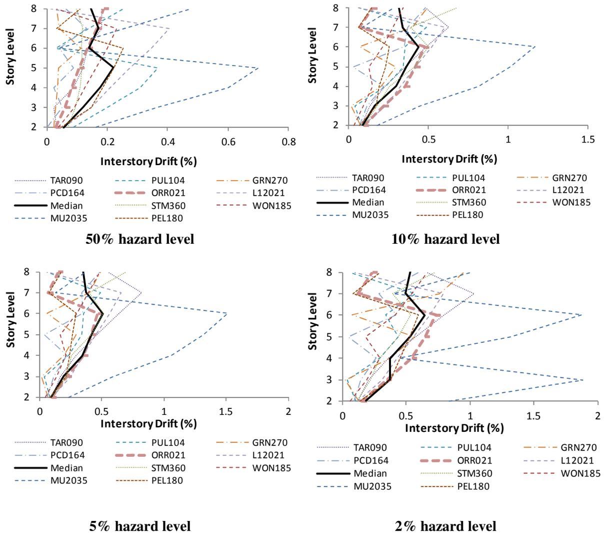
**Figure 3.10. Inter-storey drift for retrofitted case with shear wall**
