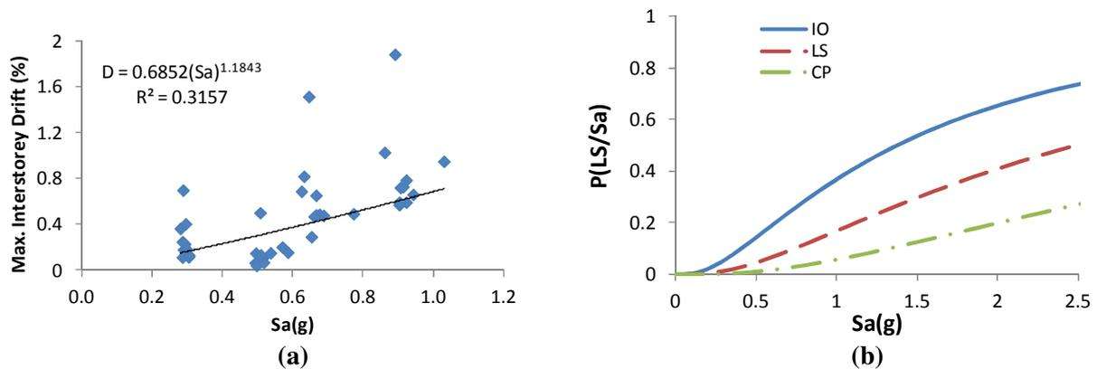
**Figure 3.15. Shear wall retrofitting, a) probabilistic seismic demand model, and b) seismic fragility curve**
