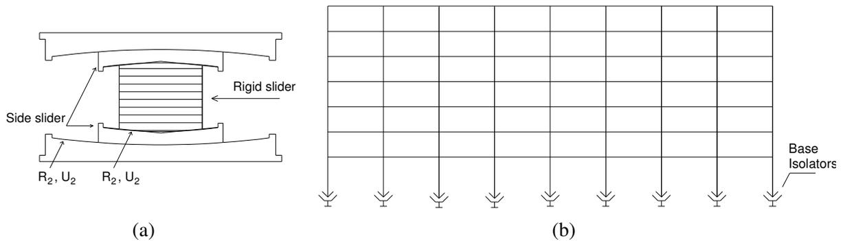
**Figure 3.4. Base isolation (a) isolator details and material property, (b) isolators added to the base of the frame**
