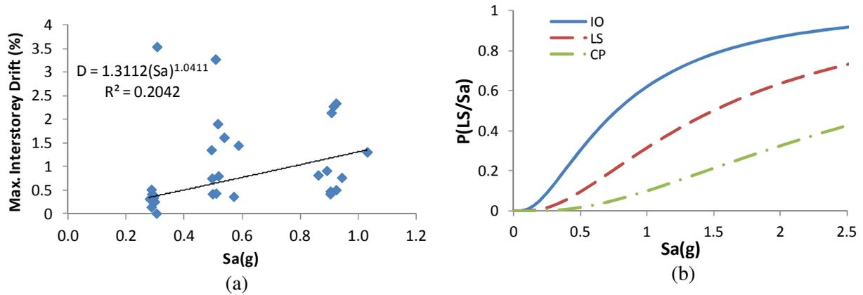
**Figure 3.16. Base isolation retrofitting, a) probabilistic seismic demand model, and b) seismic fragility curve**
