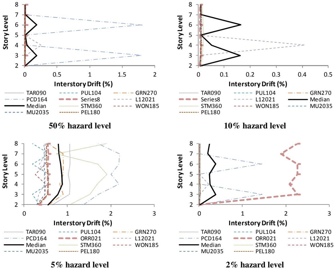
**Figure 3.12. Inter-storey drift for retrofitted case with base isolation**
