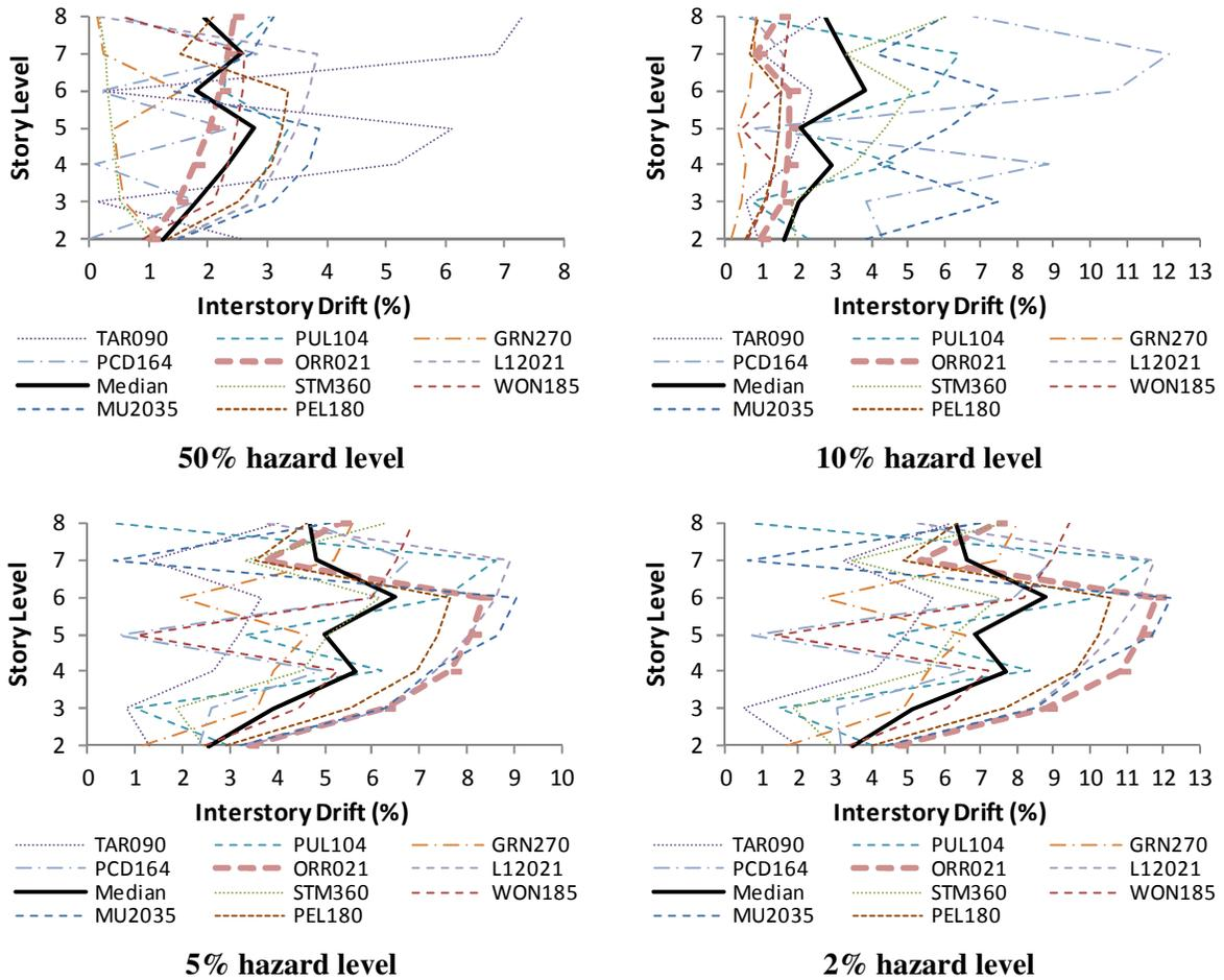
**Figure 3.8. Inter-storey drift for unretrofitted case**
