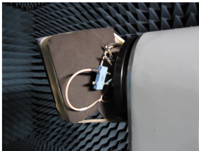
Figure 8.12: Balun Attached to the Prototype and Shielded by Radio Absorbing Material
