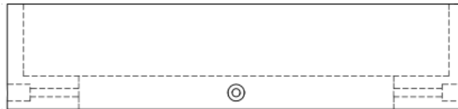
Figure 6.7: Cross Section of Choke Showing Screw Clearances
