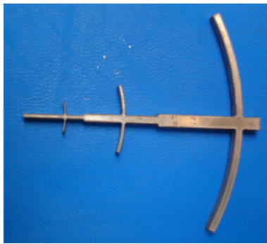
Figure 7.1: Fabricated Combined Feed Line and Excitation Elements
