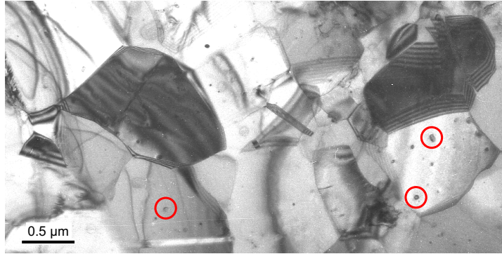
Figure 4.7: Bright field TEM image of a sample annealed for 3 minutes at 800°C resulting in a D=0.5\ \mu\text{m} average grain size, illustrating the presence of chromium nitride precipitates. Such precipitates were not found in samples annealed at higher temperatures.
