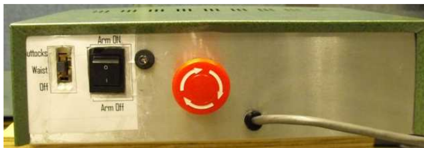
Figure C.24: Test bed control box. Use to activate the limit switches for the particular mode of rise.
