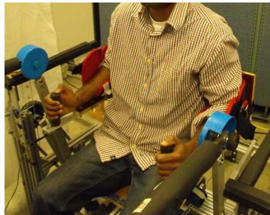
Figure C.16: Subject seated in test bed ready for arm assisted rise.
