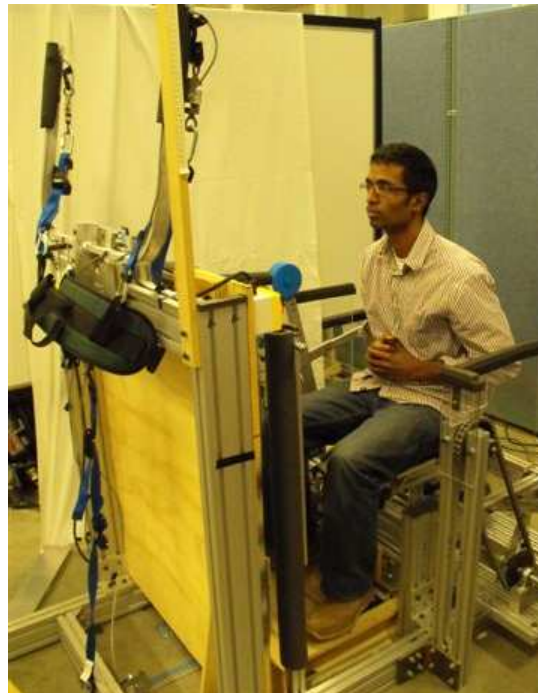
Figure C.20: Subject seated in test bed ready for buttocks assisted rise.
