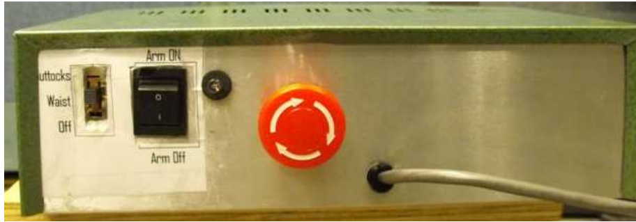
Figure 5.26: Control box. Note that the label “buttocks” on the three position selector switch represents the seat assist.
