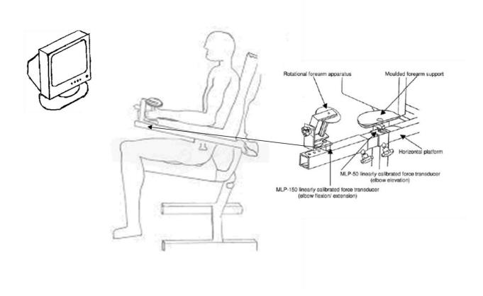
**Figure 3.1. Experimental set-up**. The left panel is a diagram of how a subject would sit during the experiment, one metre in front of a computer monitor. Elbow, hips and knees were flexed at 90°, and left shoulder was abducted at 15°. The forearm was placed in a neutral position. The right panel is a diagram of the arm apparatus. Adapted from Harwood, Edwards and Jakobi, 2010.
