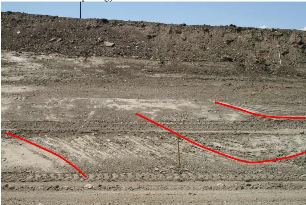
Figure 4.22: Second photo of Site F exposure taken 5 m to the north of Figure 4.21. Undulating silt beds outlined in thick red line to show the morphology. Meter stick for scale.
