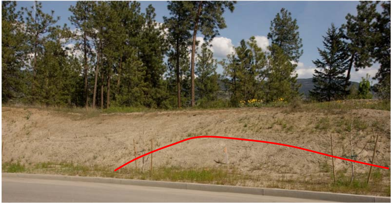
Figure 4.30: Photo of undulating silts adjacent to Seismic line 00-02. The thick red line indicates the separation of upper laminated silts from lower massive sands.
