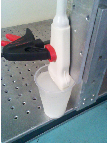
Figure 4.1: The experimental setup used for the experiments of this section. The ultrasound probe is dipped into the water layer on top of the phantom, and clamped to a metal strut on an anti-vibration table.
