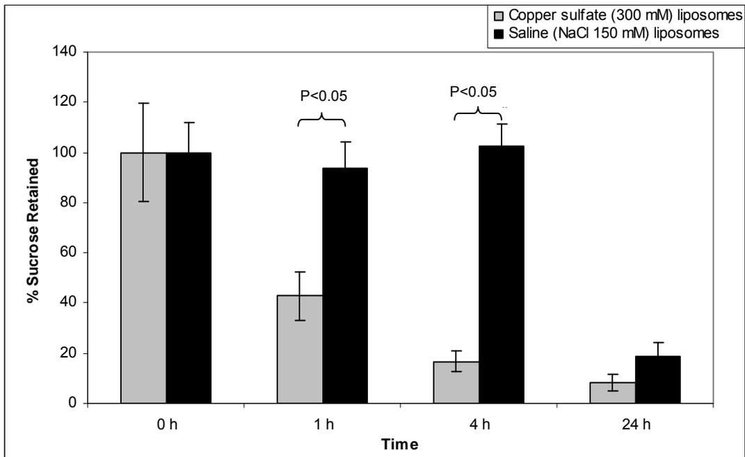
**Figure 2.7:** Membrane permeability study of DSPC/CH liposomes: Liposomes prepared using either copper sulfate (300 mM) or saline (NaCl 150 mM) were kept in 70°C water bath. Amount of <sup>14</sup>C-labeled sucrose retained inside the liposomes was measured by passing the aliquots through a sephadex G-50 spin column equilibrated with PBS. Data points represent the mean ± SD (n=3).
