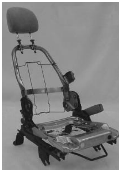
Figure 1-5: GM High Retention Seat frame structure (adapted from [25])
