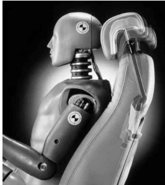
Figure 1-4: Self-Aligning Head Restraint (SAHR - adapted from [2])
