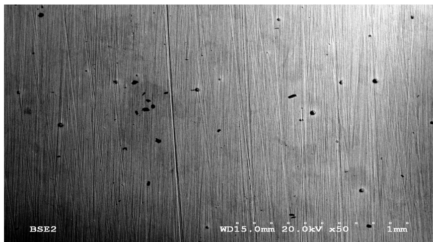
Fig. 5.11 SEM morphology for the magnesium surface layer after the test.
