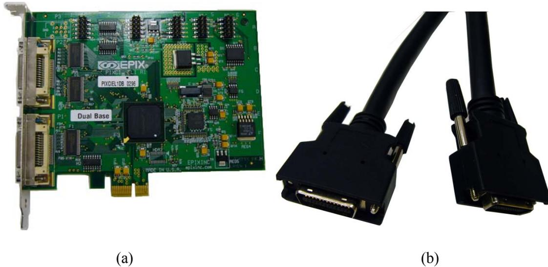
**Figure 2.7:** (a) Frame grabber (PIXCI® EL1DB from EPIX); (b) Camera link cable.
