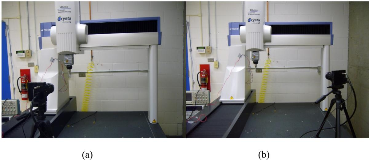
**Figure 5.13:** (a) Camera setup for the left view; (b) Camera setup for the right view.
