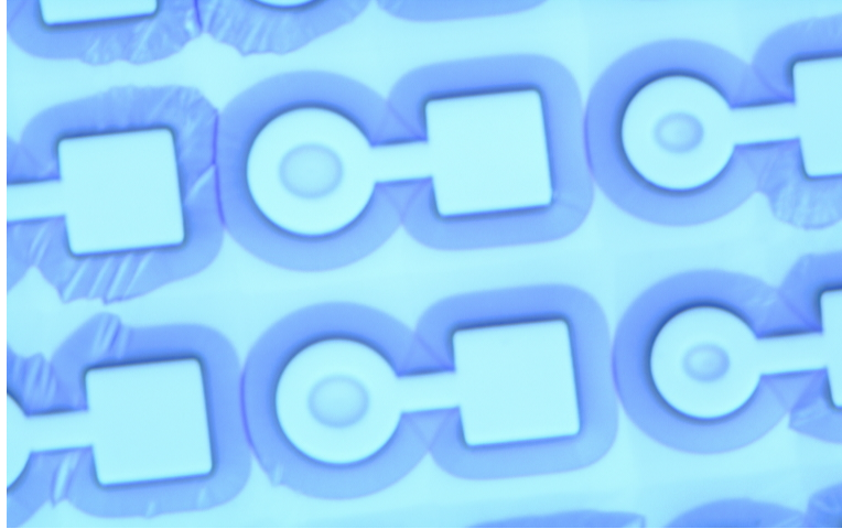
Figure 3.12: 3\text{H}_2\text{SO}_4 : \text{H}_2\text{O}_2 : \text{H}_2\text{O} system is highly corrosive (etch rate mainly proportional to Sulphuric acid concentration) and results in large amount of undercut. Not suitable for our masking patterns.
