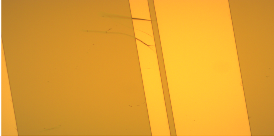
Figure 3.10: Defect revealed after developing due to presence of impurities in the PR. This problem was resolved by using fresh PR and also ensuring that the sample surface was cooled before PR spinning.
