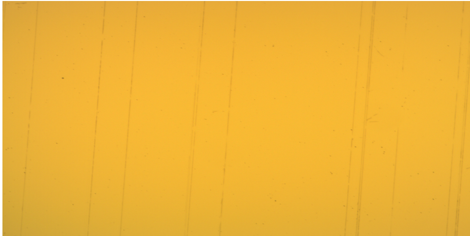
Figure 3.11: PR residue left over after cleaning including the following approaches: over-flooding the PR with the UV and developing, two-solvent process at room temperature, two-solvent process at close to boiling temperature. This is most likely due to expired PR and/or over-baking the PR. A PR stripper solution can usually remove the residues.
