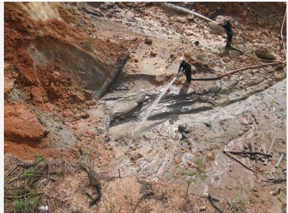
2 – Use of hydraulic monitors in sensitive areas
