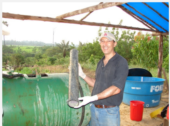
4 – Activated charcoal in a perforated tube
