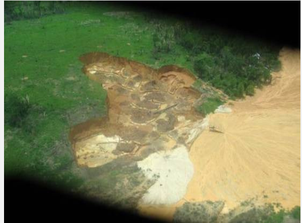
2 – Pit is open and tailings released into the rivers
