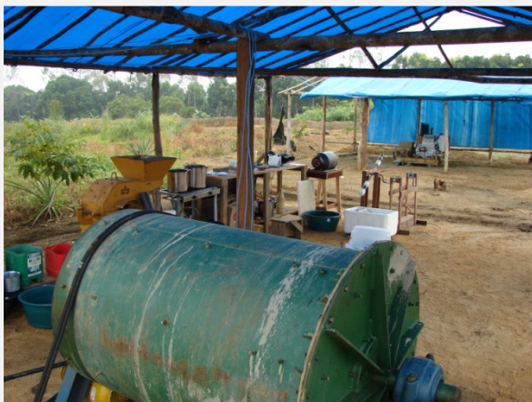
5 – Cyanidation in ball mill in progress
