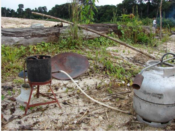
1 – Use of retorts to burn amalgam in the field
