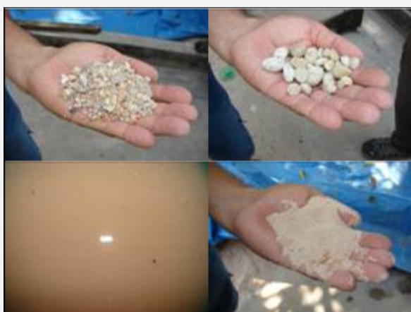
5 – Layers of pebbles, sand and biofilm
