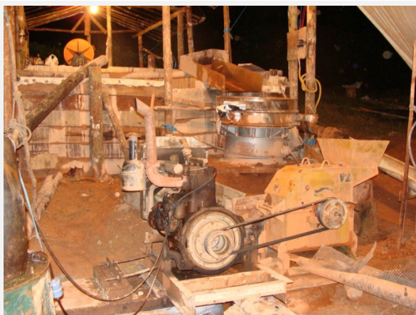
2 – Internal view of sieve and hammer mill
