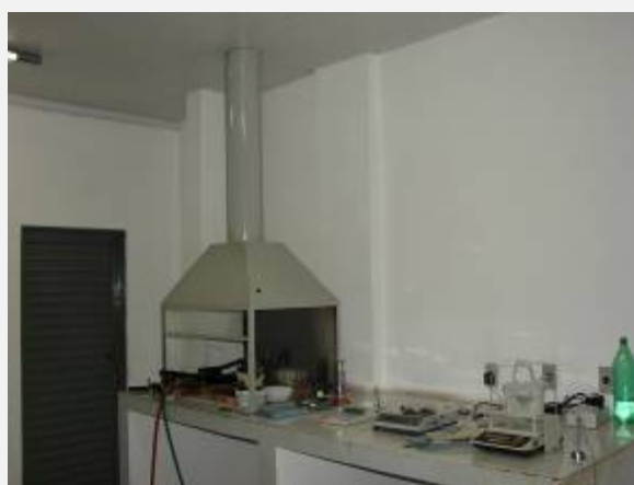
3 – Gold shop and chamber without mercury filter
