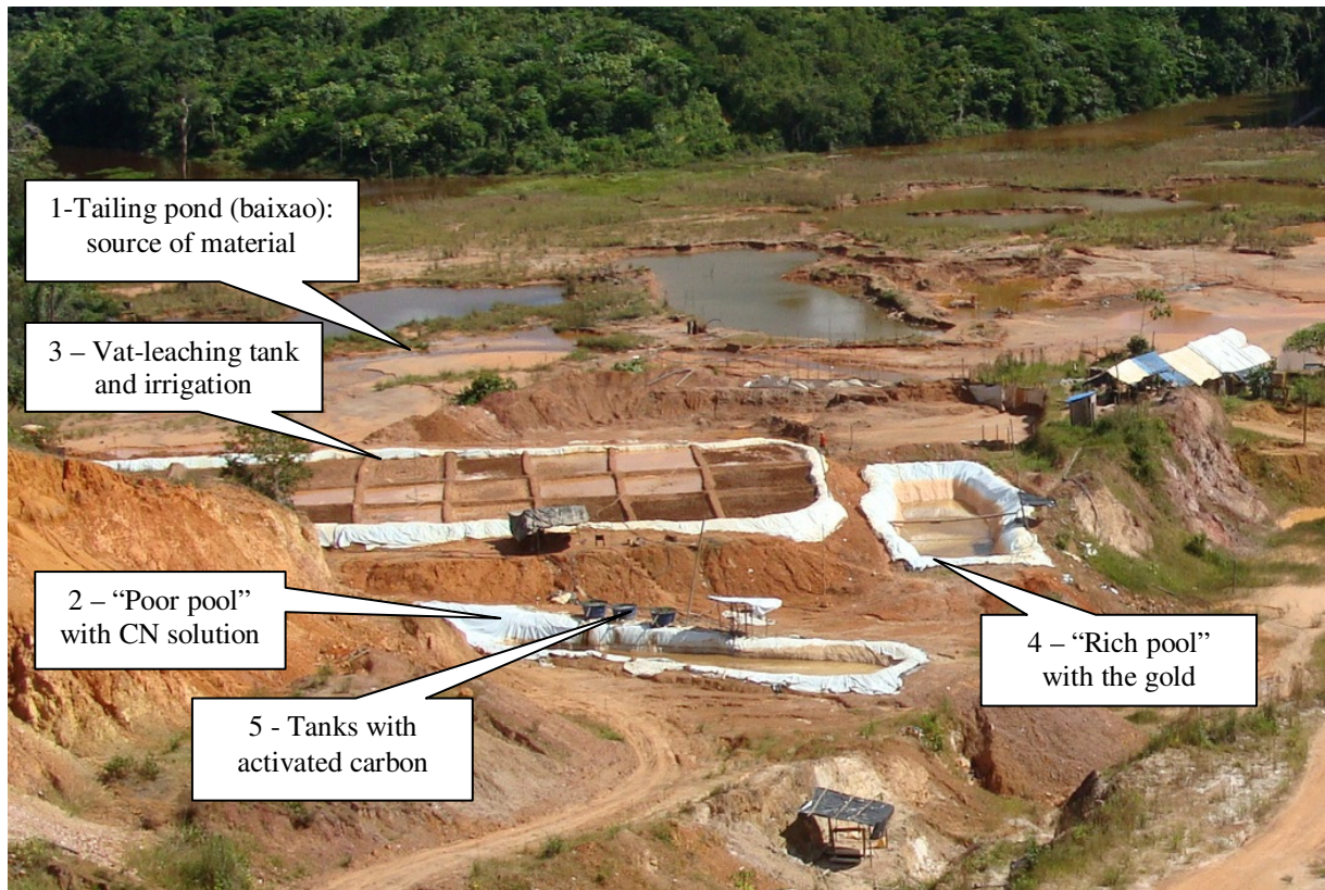
Figure 5-4 – General view of the vat-leaching process
