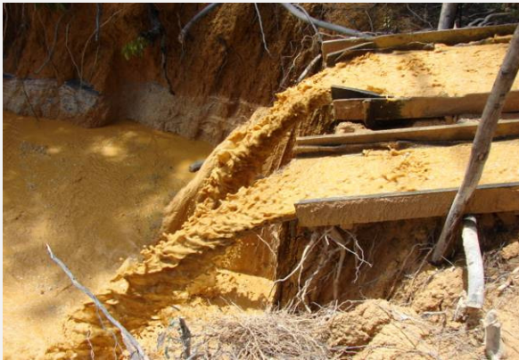
3 – Tailings redirected to refill old pits
