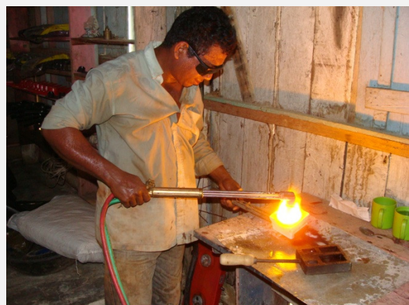
6 – Smelting after retort
