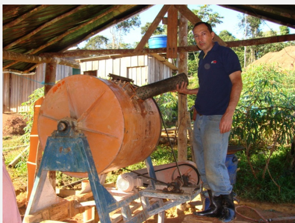
4 – Capsule of activated carbon in the ball mill
