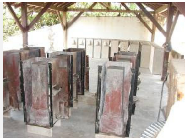
2 – Cement biosand filters under fabrication
