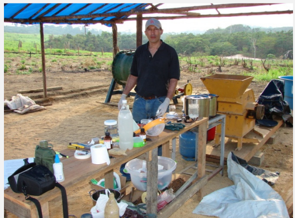
6 – Gold recovery by zinc precipitation
