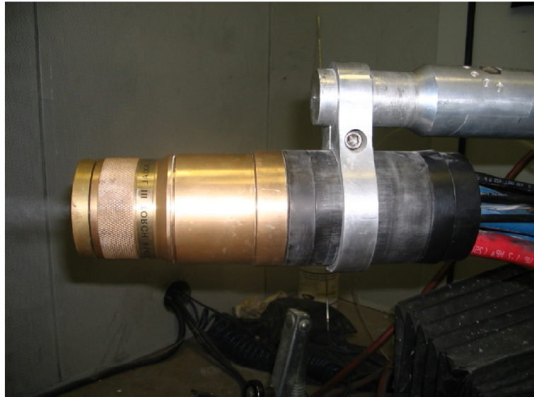
Figure D.5: Image of the two fluid atomizing nozzle suspension injection system in operation (no plasma).
