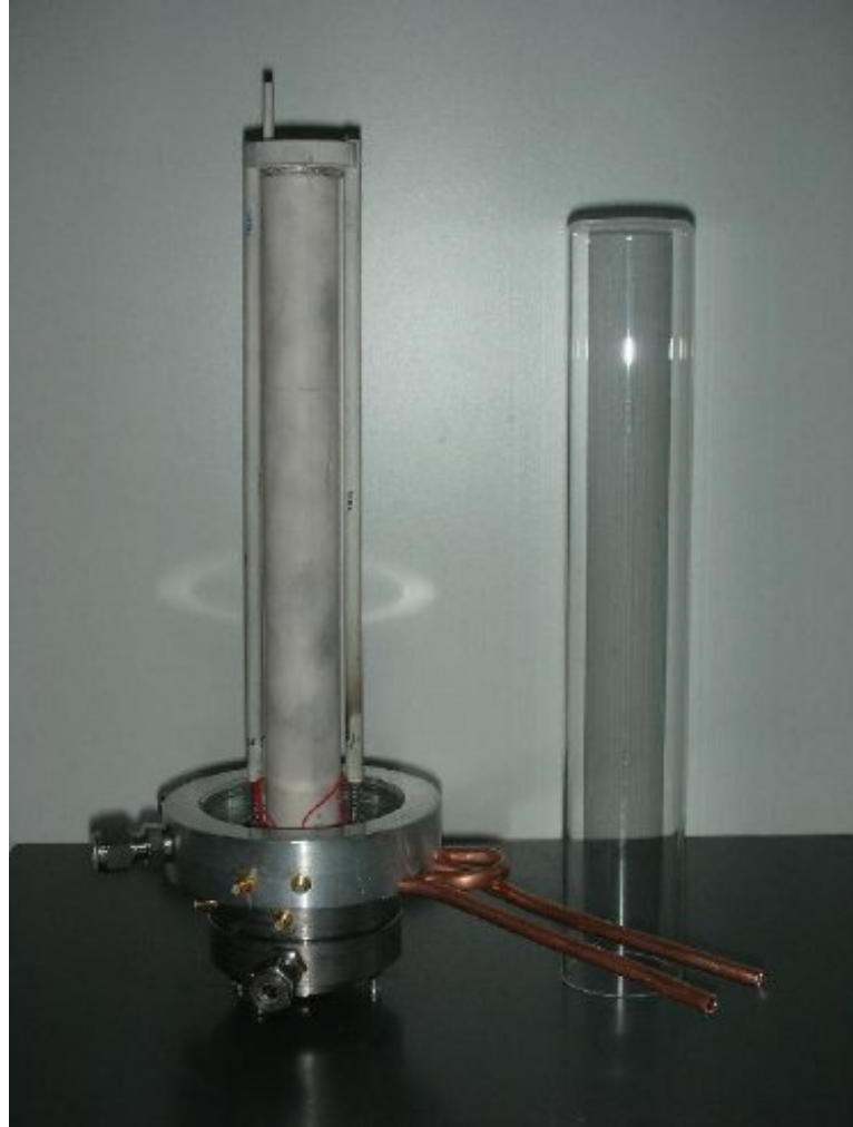
Figure E.1: Single cell test station fixture [1].
