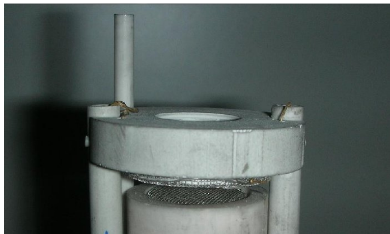
Figure E.2: Test station fixture contact area [1].
