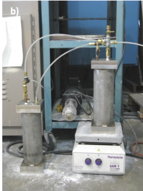
Figure 4.2: a) Mettech Axial III plasma spray torch. b) Pressure vessel based suspension delivery system.
