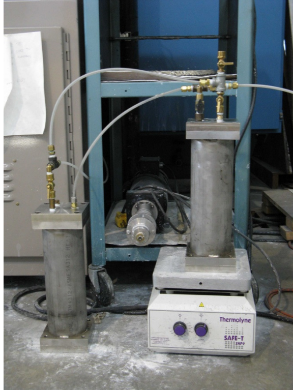
Figure D.2: Image of the pressurized canister delivery system.
