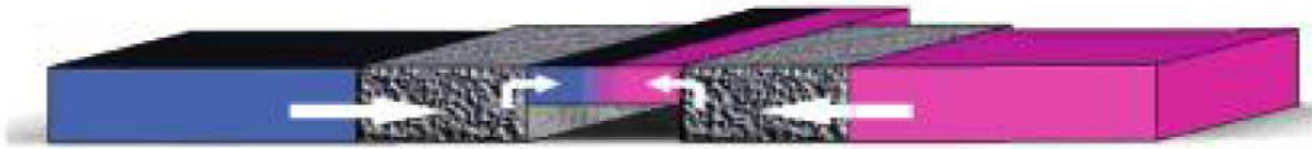
Figure 1.11 The schematic of the microfluidic fuel cell with flow-through porous electrodes fabricated by Kjeang et al. [36]
