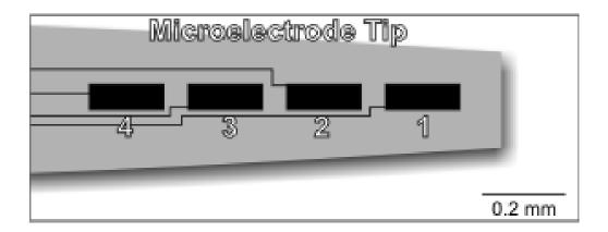
The microelectrode array consists of four  $\sim 200 \times \sim 50$  micron Pt recording sites. All four recording sites are coated with Nafion<sup>®</sup>. Only site 1 is additionally coated with glutamate oxidase.
