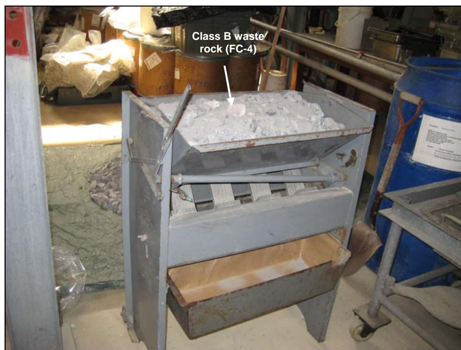
Figure 3.2 Riffing by using the Gilson Splitter Model SP-1 of Class B waste rock samples before starting the laboratory testing
