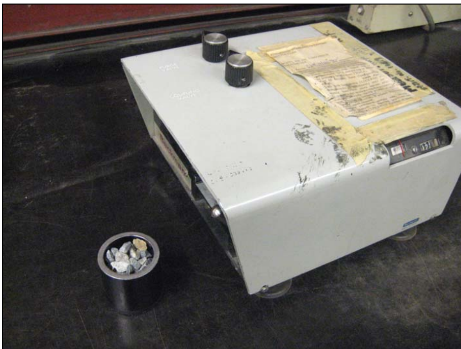
Figure C6.5 Air comparison pycnometer in determining volume and density particle of waste rock material
