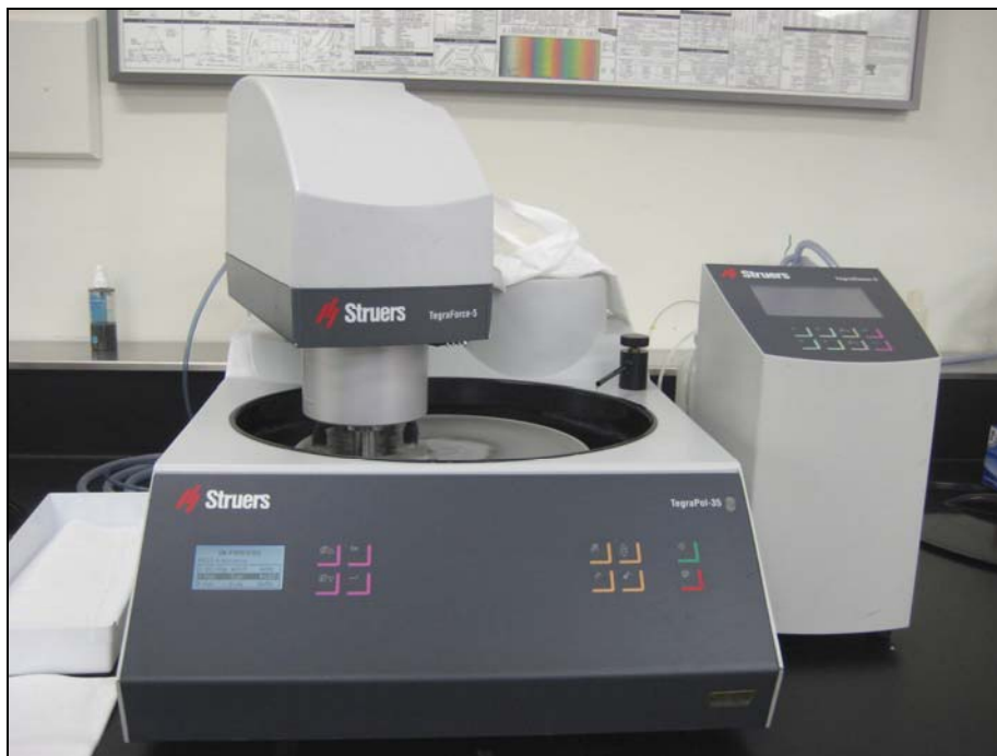
Figure C6.10 Struers Tegra polisher system for polishing mounts to analyze with MLA
