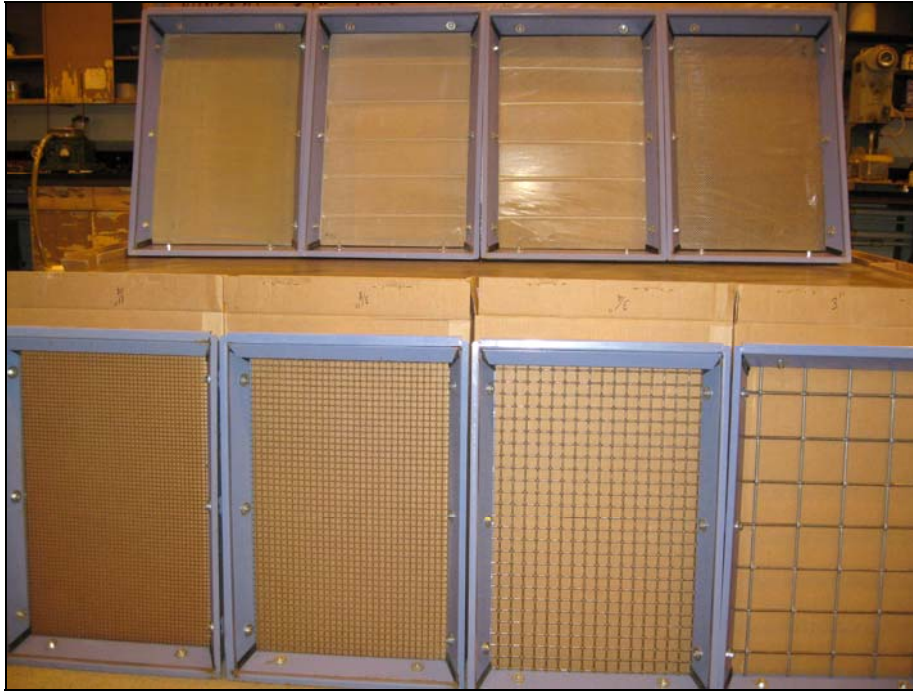
Figure C6.1 The US Standard Sieve Trays (45 cm x 65 cm) for wet particle size analysis of coarse size fractions
