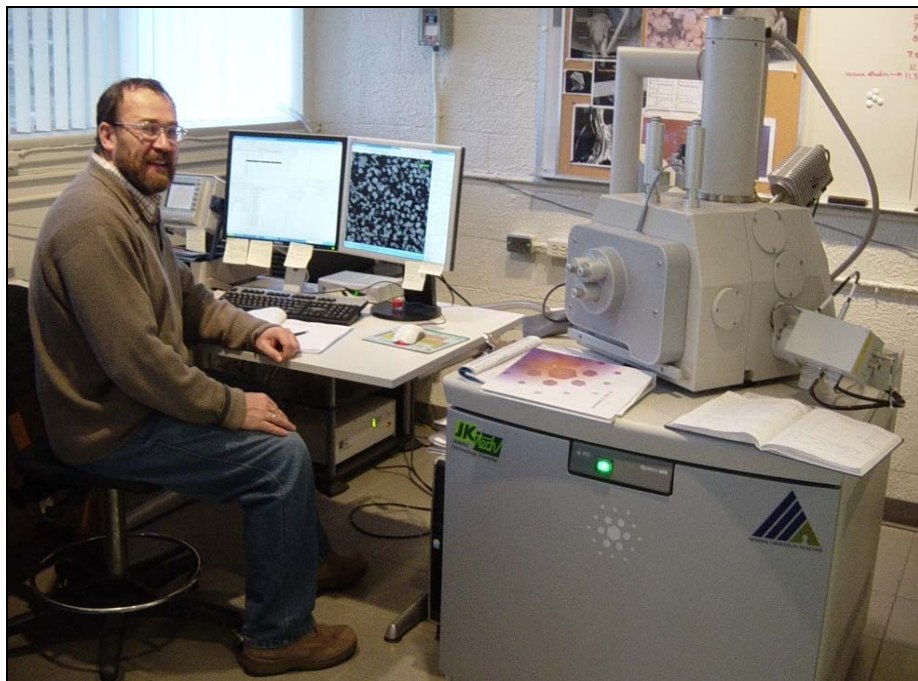
Figure C6.12 FEI Quanta600-SEM Mineral Liberation Analyzer (MLA) of Teck's ART group at Trail, B.C.
