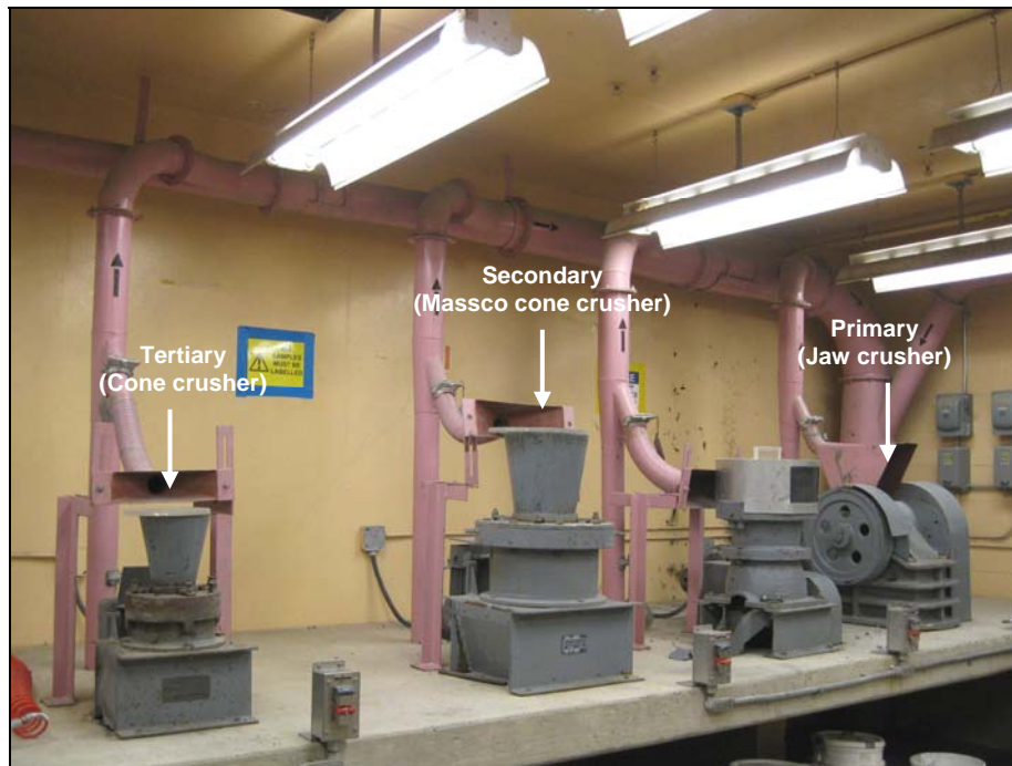
Figure C6.7 Crushers used during the coarse size fractions grinding for preparing samples for assay
