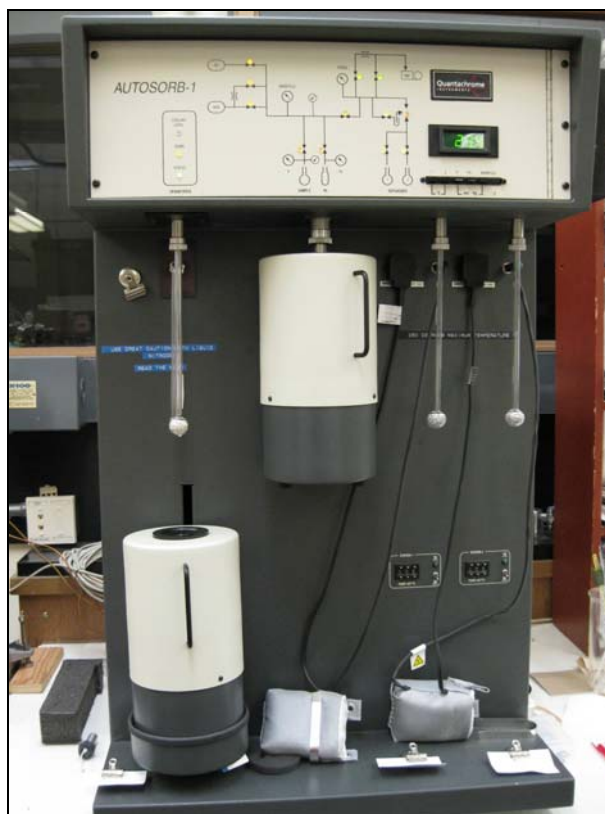
Figure C6.6 Autosorb-1 Surface Area Analyzer (Quantachrome Instruments Corporation) for determining specific surface area by using the BET method
