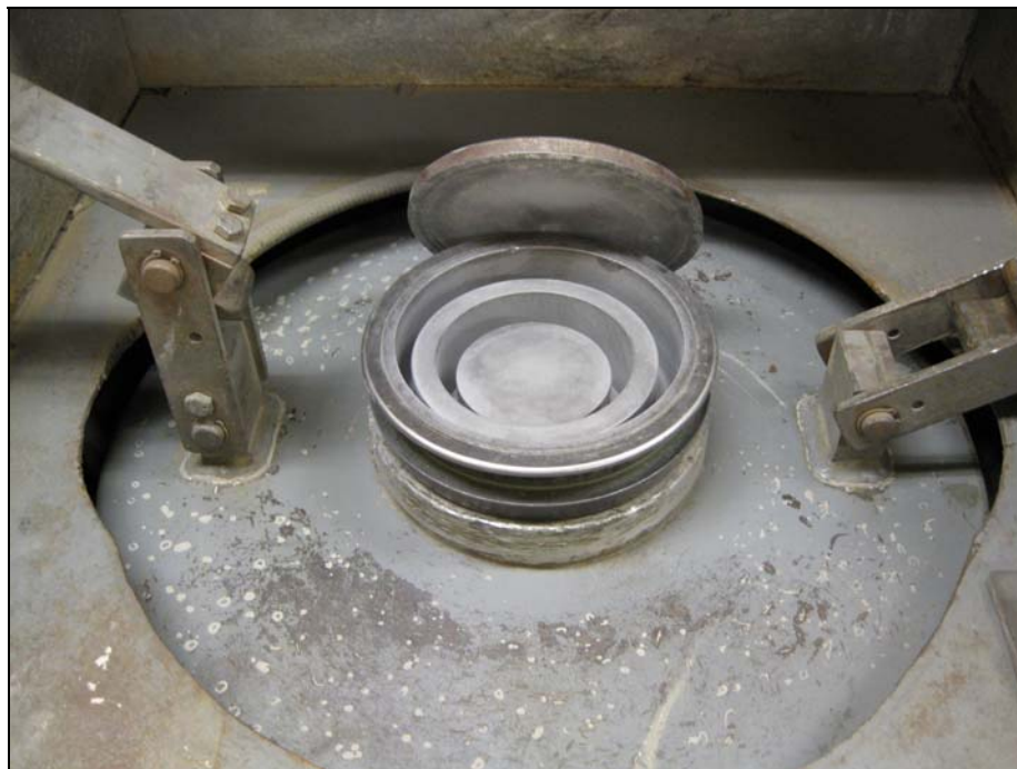
Figure C6.8 Ring mill pulveriser using a carbon steel (chrome free) ring set (TM Engineering Ltd.) for preparing samples for assay
