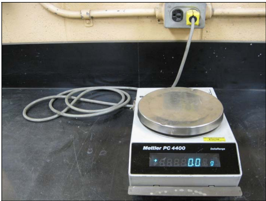
Figure C6.4 Laboratory scale (Mettler PC 4400) using for particle size analysis and sample preparation for assay
