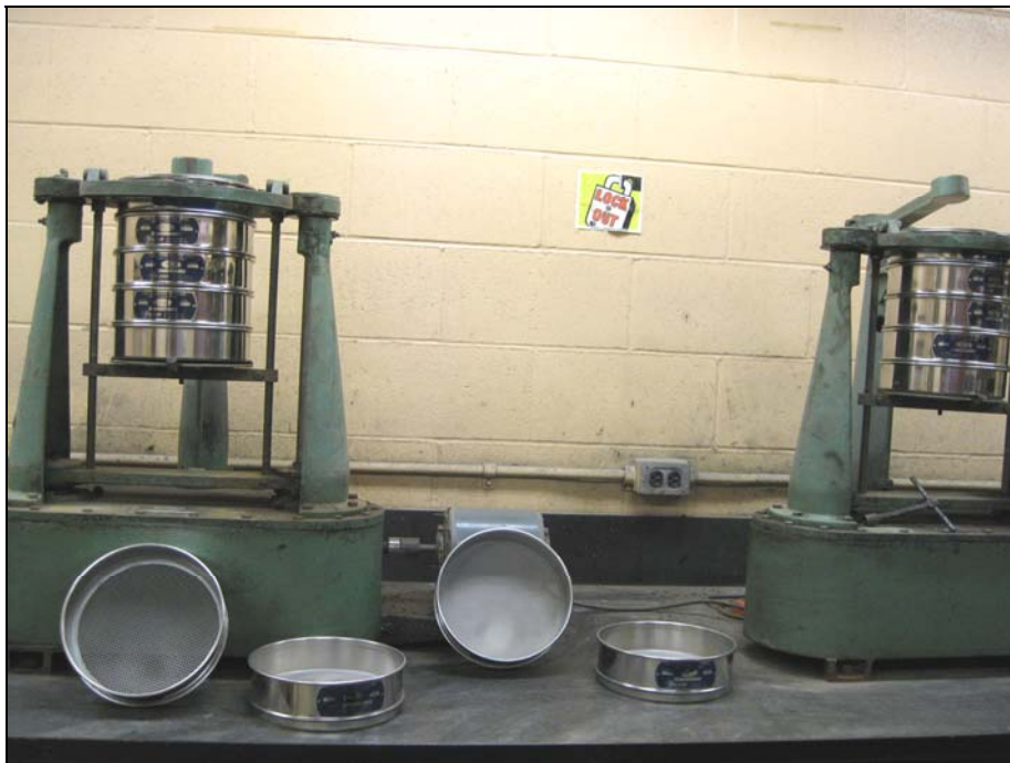
Figure C6.2 Eight-inch standard round Gilson stainless steel cloth sieves in vibrating shakers (ro-taps) for dry particle size analysis of fine size fractions
