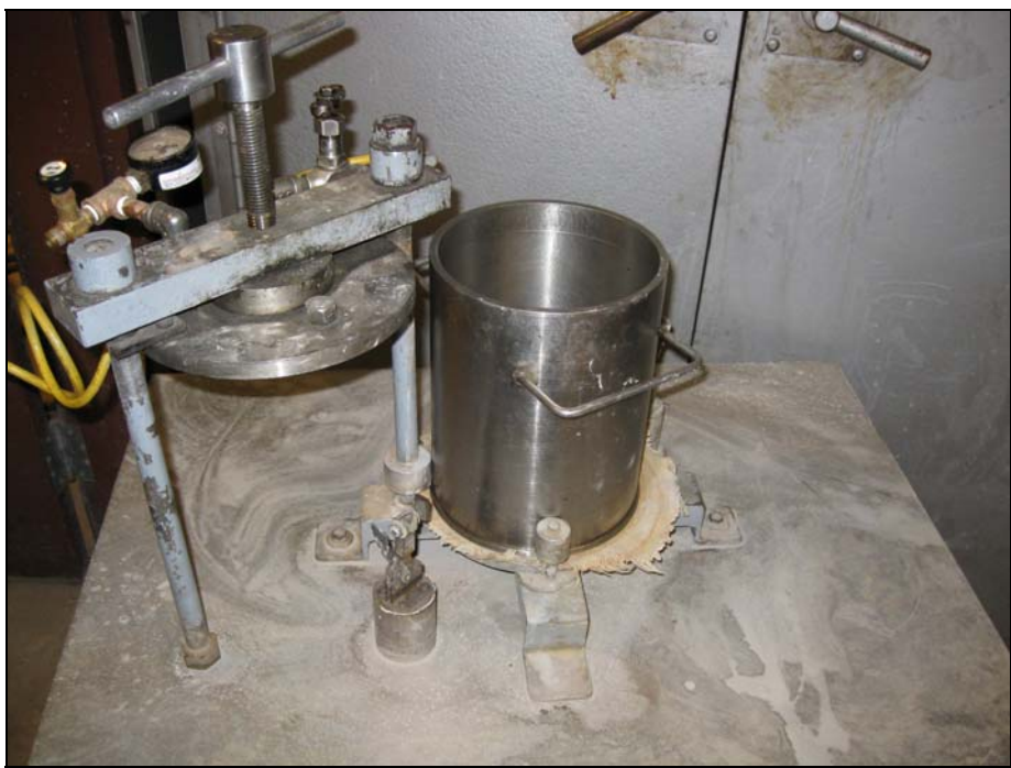
Figure C6.3 Pressure filter for filtration of finest particles during the particle size analysis
