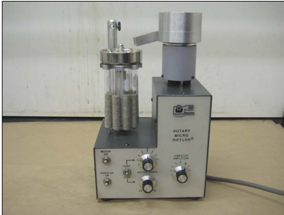
Figure C6.9 Rotary micro riffler with 3 inch turntable, 15mm OD x 8 tubes (Quantachrome Instruments Corporation) for preparing samples to analyze with MLA
