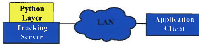
Figure 3.12: Communication Diagram. The tracking program acts as a server wrapped in Python, and the user study application is a client that receives commands and sends data to the server.
