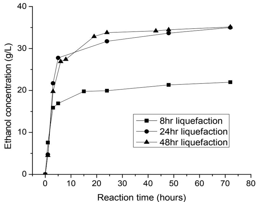
Figure 5-14. Fed-batch LSSF at different liquefaction time.
