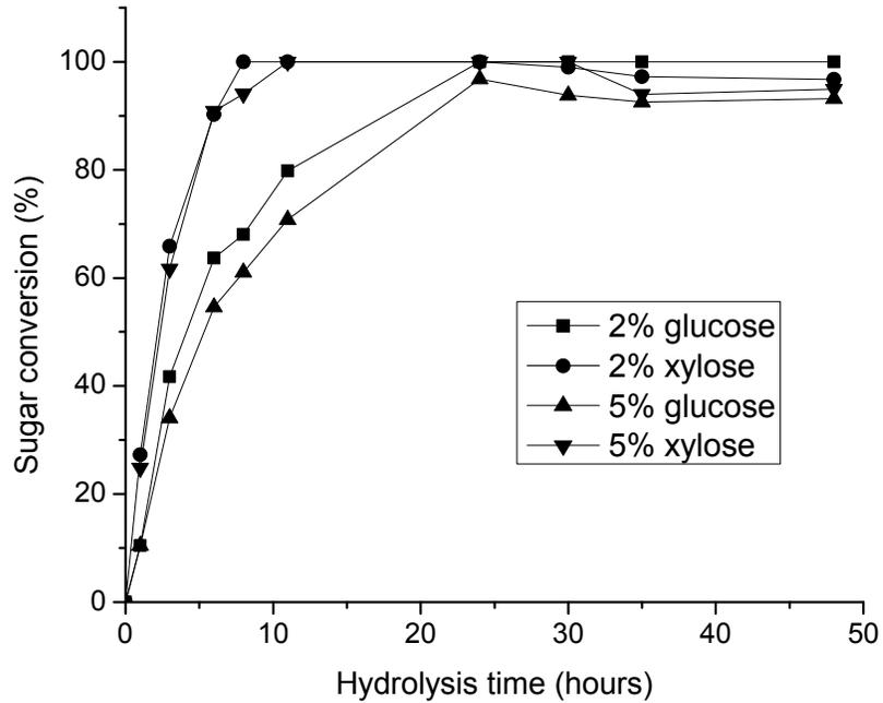
Figure 4-1. Enzymatic hydrolysis of UBHW at 2% and 5% substrate consistencies in shake flasks at 20FPU/80CBU/g of cellulose enzyme loading, based on A) glucose and xylose concentration formed and B) percent sugar conversion.
