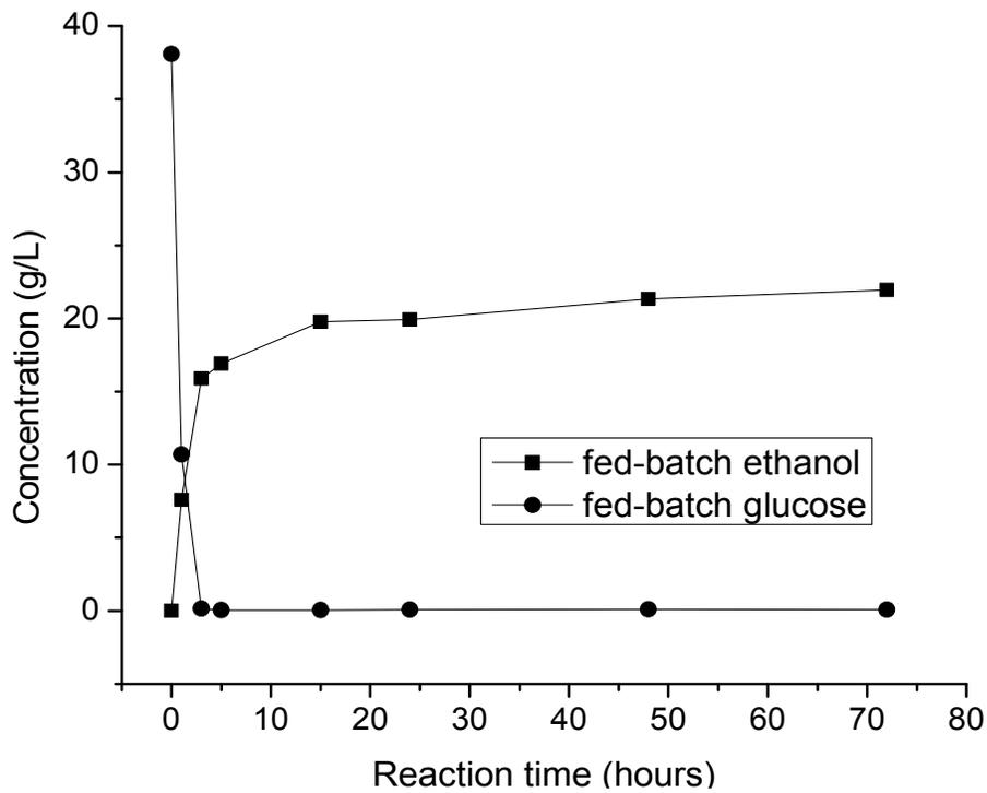
Figure 5-13. Fermentation of hydrolysate from fed-batch hydrolysis.
