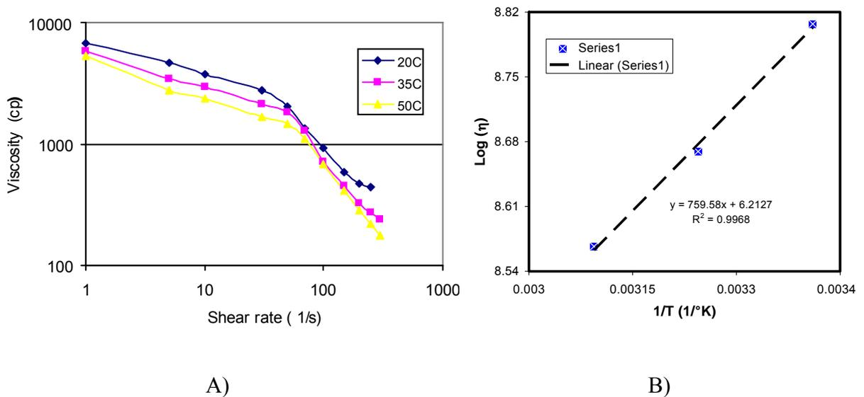
Figure 3-5. A) Viscosity of hydrolysate versus shear rate under various temperatures. B)  $\log \eta$  versus  $1/T$  fitting by Arrhenius equation.
