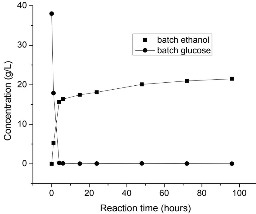
Figure 5-12. Fermentation of hydrolysate from the single-batch hydrolysis.
