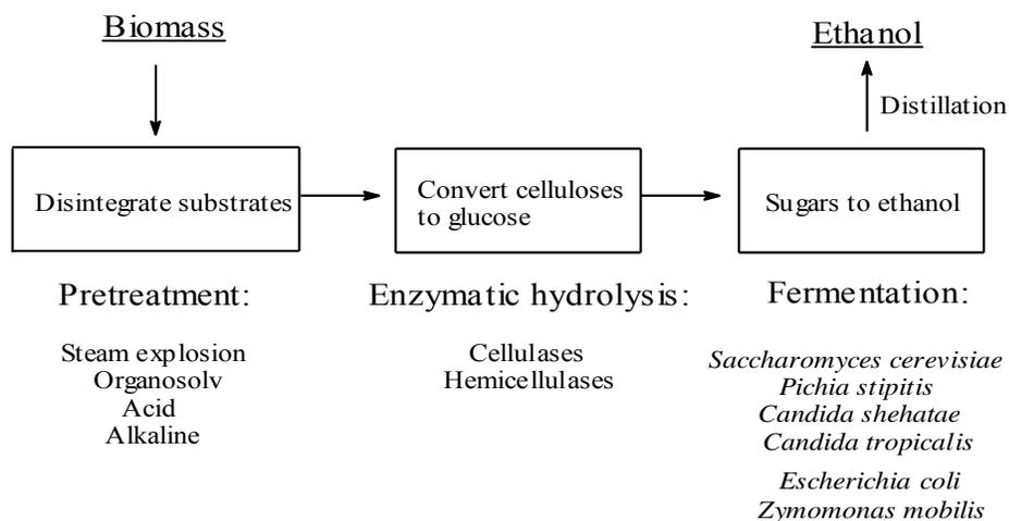
Figure 1- 1. Schematic diagram of a bioconversion biomass-to-ethanol process.
