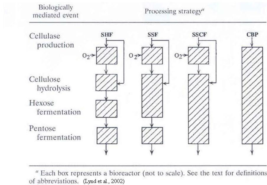
Figure 1- 2. Evolution of biomass-processing schemes featuring enzymatic hydrolysis
