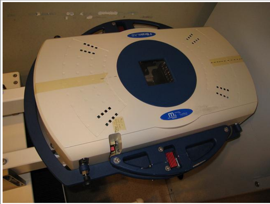
Figure 4.7: This is a photograph of the BrainLAB m3 micro MLC. This device is attached to the gantry head when in use. The square window in the center is where the beam passes through. Noticeably the maximum field size is only 10 cm by 10 cm defined at 100 cm distance. The leaves can be seen on the right edge inside of the window.
