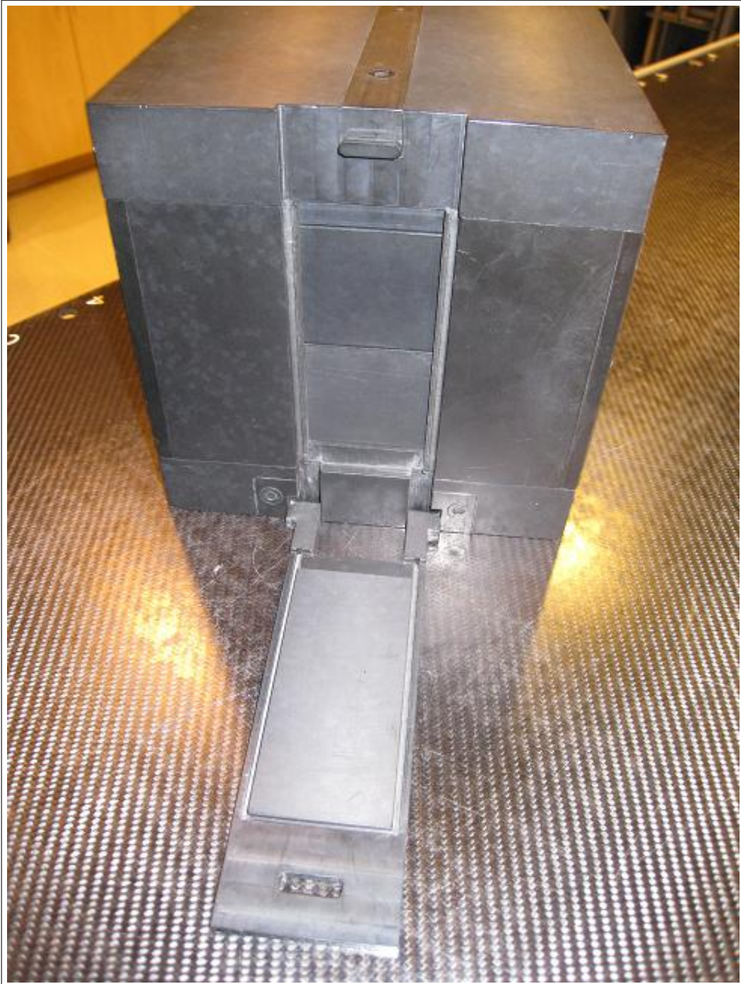
Figure 3.8: Part of the film cube phantom is opened showing the internal structure.
